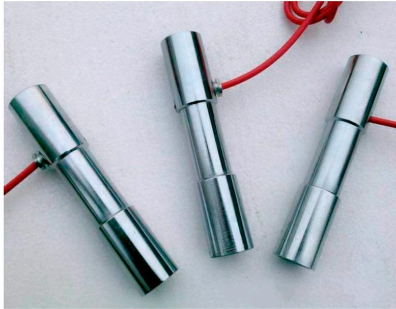
**Figure 5.** Rebar stress gauge.
