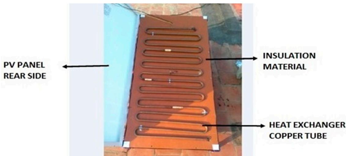
**Figure 3.** Pictorial view of copper tube along with a solar panel.
