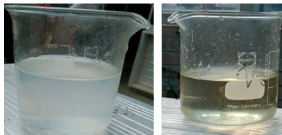
Figure 6. Before 'B' (influent) and After 'A' (effluent) samples of GW were examined for water testing parameters.
