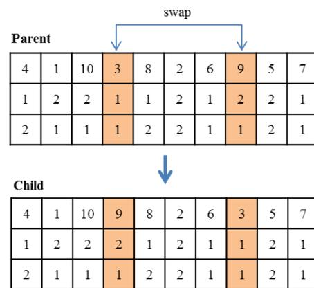
**Figure 6.** Illustration of Mutation\_1 for  $\pi(1)$ .
