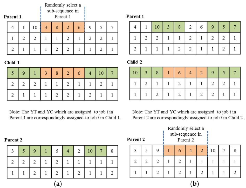
Figure 4. Illustration of the order crossover for  $\pi(1)$ . (a) Generation of Child 1, (b) Generation of Child 2.
