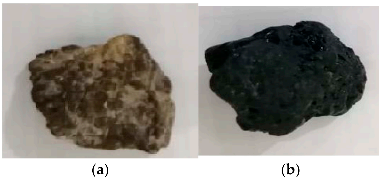
Figure 14. Aggregate visual inspection: (a) natural aggregate; (b) plastic aggregate.
