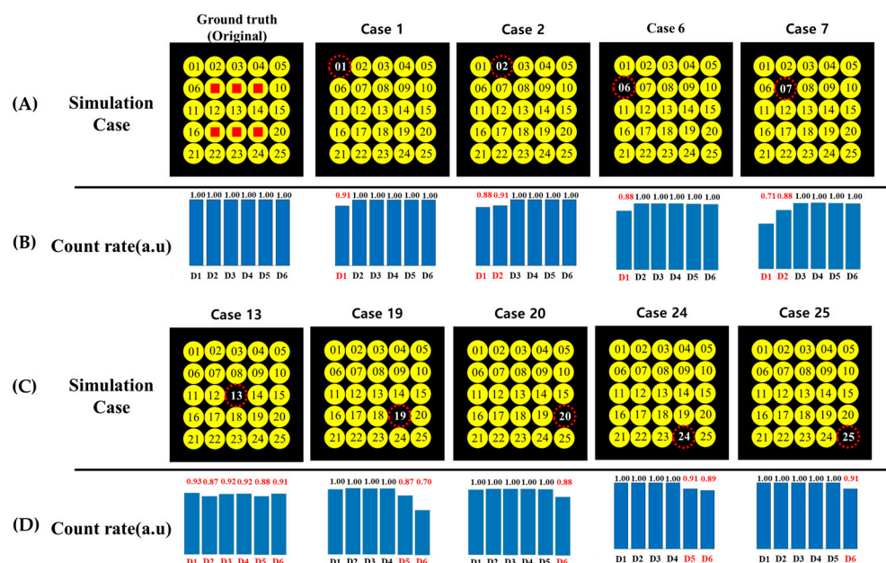
Figure 7. Simulation cases of one drum removal (A,C) and count rate comparison of each detector module (B,D).
