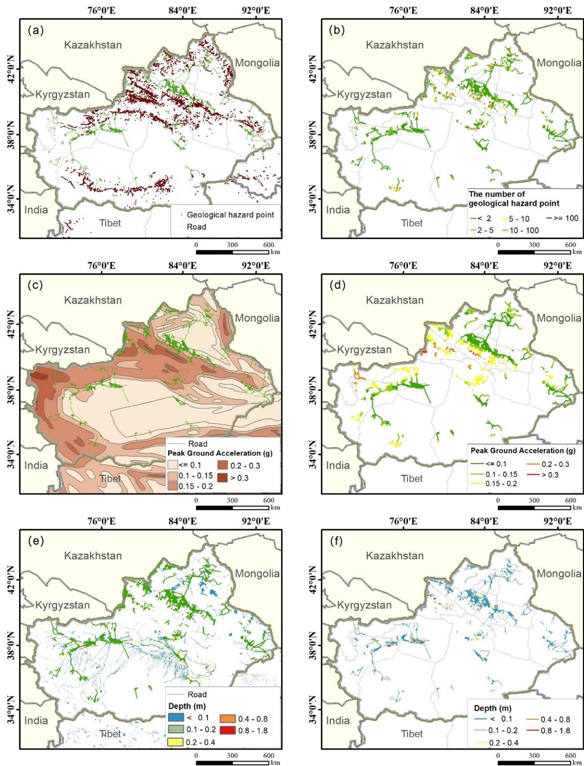
**Figure 4.** (a) The spatial distribution of the geological hazard points, (b) geological exposure map of the highway, (c) the spatial distribution of earthquakes, (d) earthquake exposure map of the highway, (e) the spatial distribution of floods, and (f) flood exposure map of the highway.
