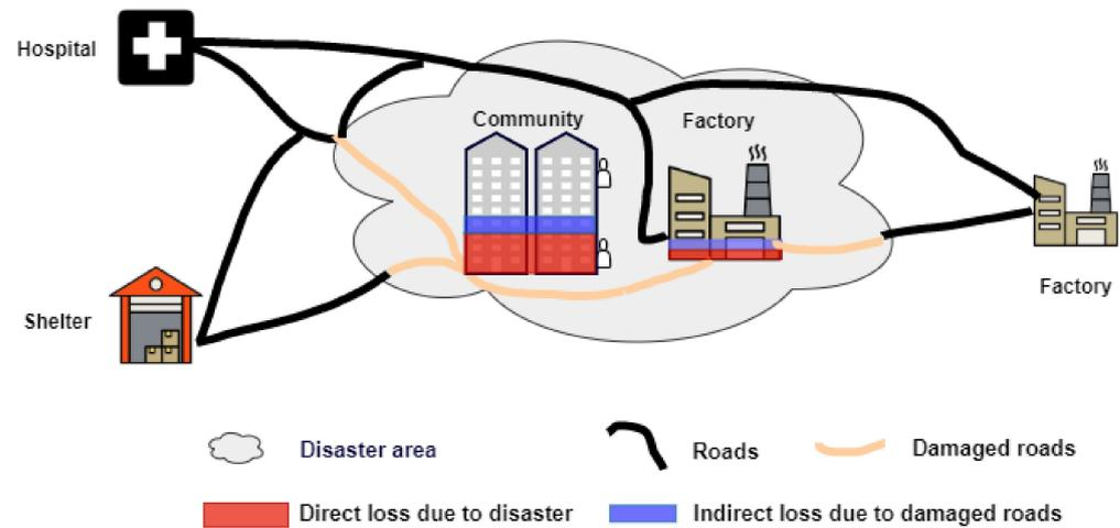
**Figure 1.** Impacts due to natural hazards and damaged roads. In the disaster area (grey), the community and factory will be affected immediately when the disaster occurs (red presents direct loss for the community and factory due to a disaster). After the disaster, indirect losses may occur since aggravated injury due to untimely rescue and supply to the disaster area is hampered (blue is the indirect loss for the community and factory due to damaged roads).
