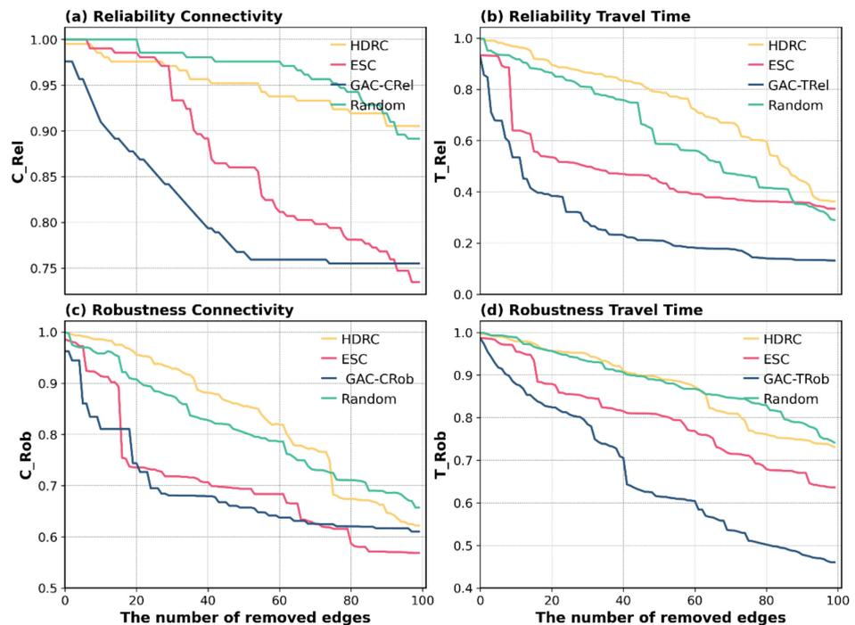
**Figure 6.** Relative reliability and robustness metrics change for highway network under different attack strategies, (a) reliability connectivity, (b) reliability travel time, (c) robustness connectivity, and (d) robustness travel time.
