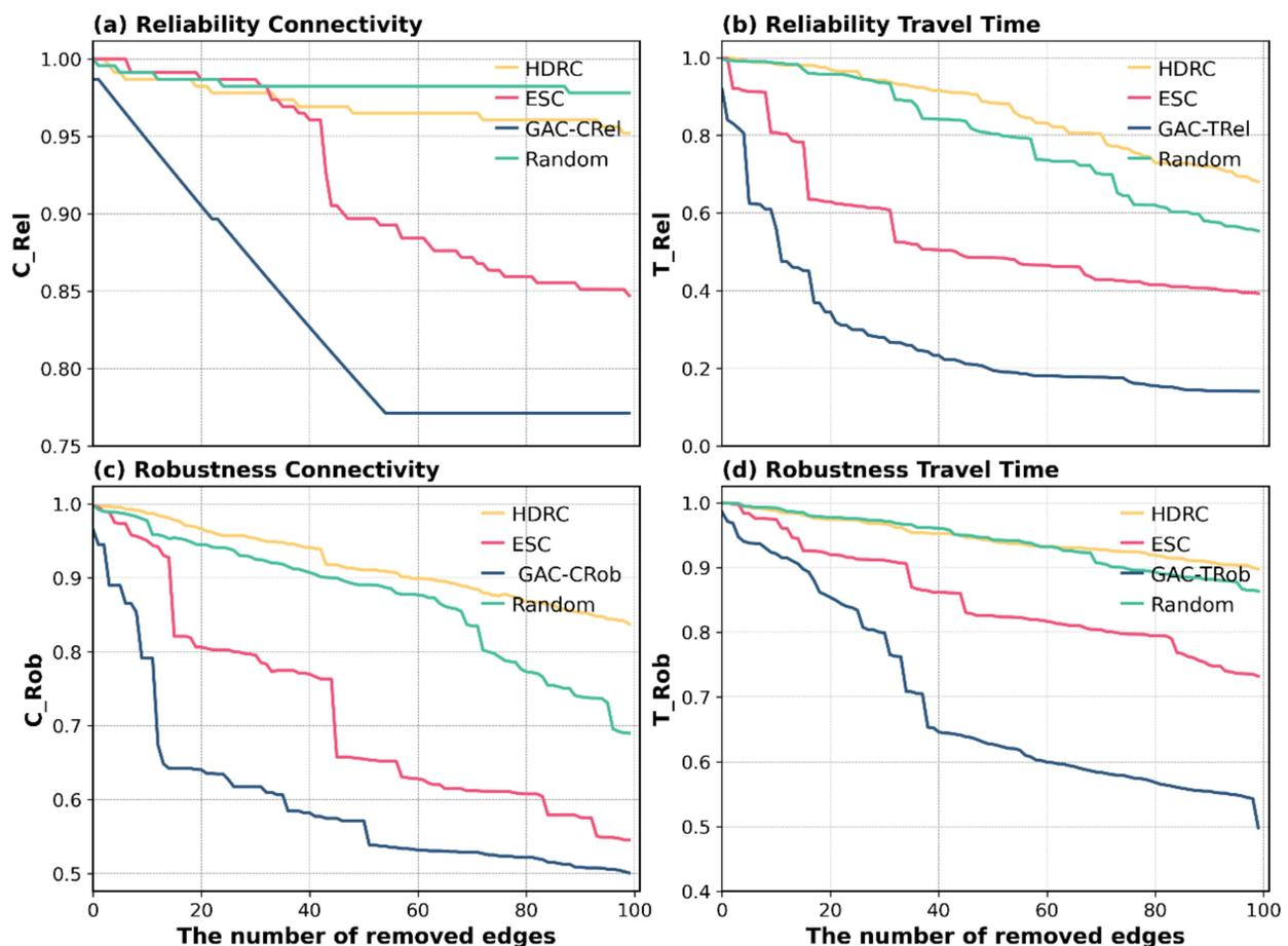
**Figure 7.** Relative reliability and robustness metrics changes for the planned highway network under different attack strategies, (a) reliability connectivity, (b) reliability travel time, (c) robustness connectivity, and (d) robustness travel time.
