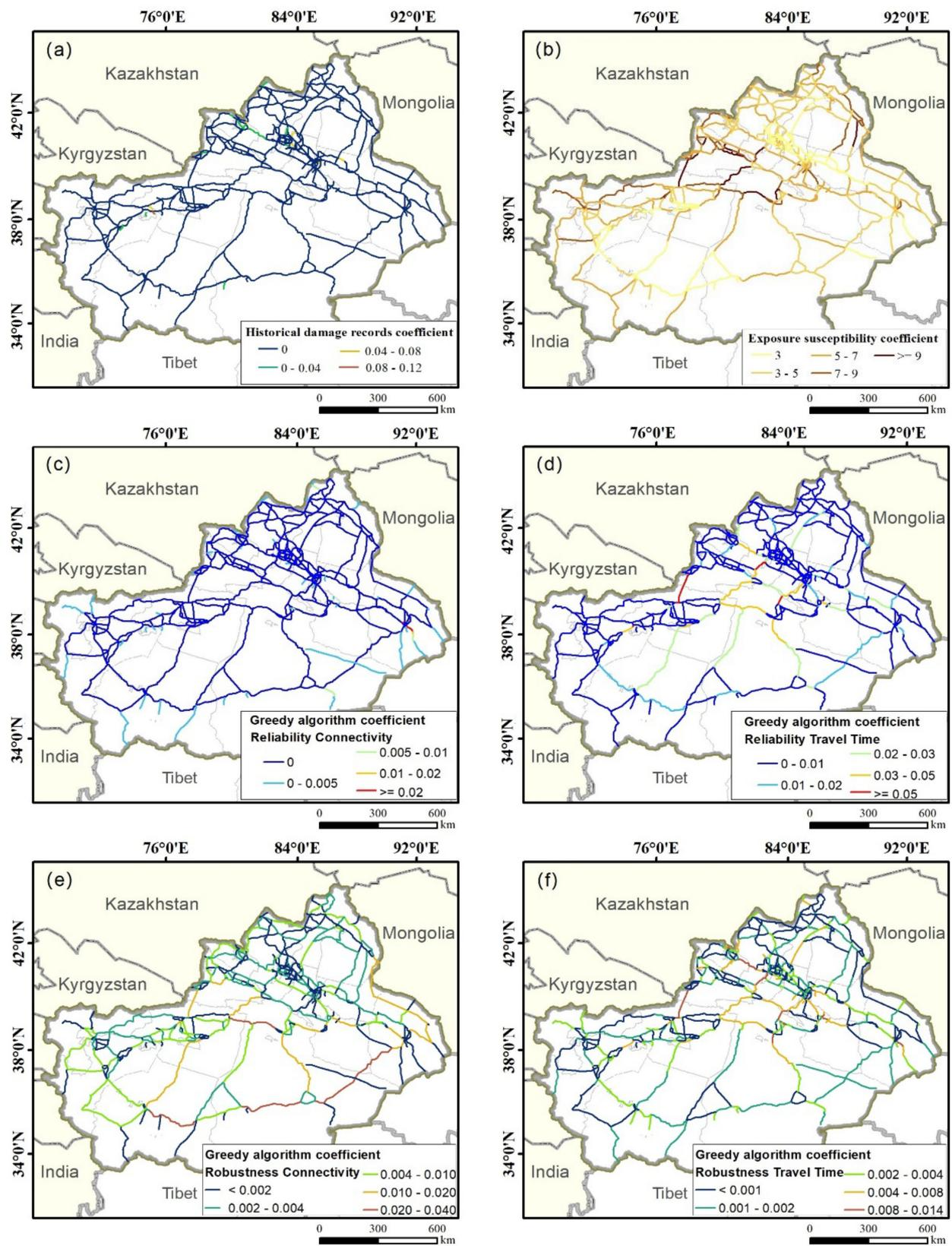
Figure 5. Spatial distribution of the influential edges in the arterial highway network using the (a) HDRC, (b) ESC, (c) GAC-CRel, (d) GAC-TRel, (e) GAC-CRob, and (f) GAC-TRob strategies.
