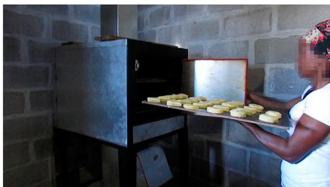
**Figure 4.** Baking of scones with the improved biomass oven by trained BREADrev facilitators in Dunoon.
