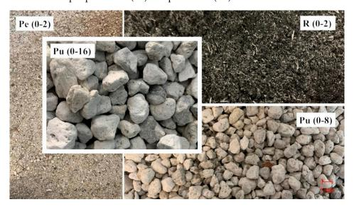
Figure 1. Lightweight aggregates.
