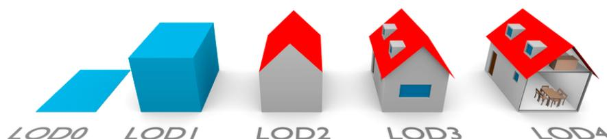
**Figure 3.** Level of Detail (LOD) on standard CityGML (source: [78]).
