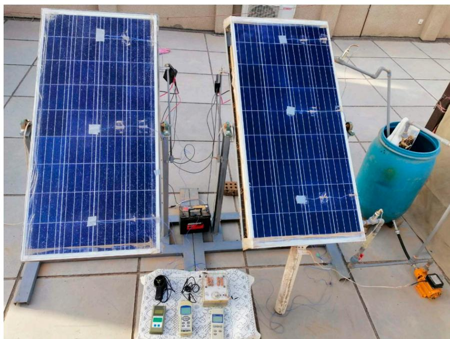
**Figure 2.** Experimental setup of the PV and PV/T system.
