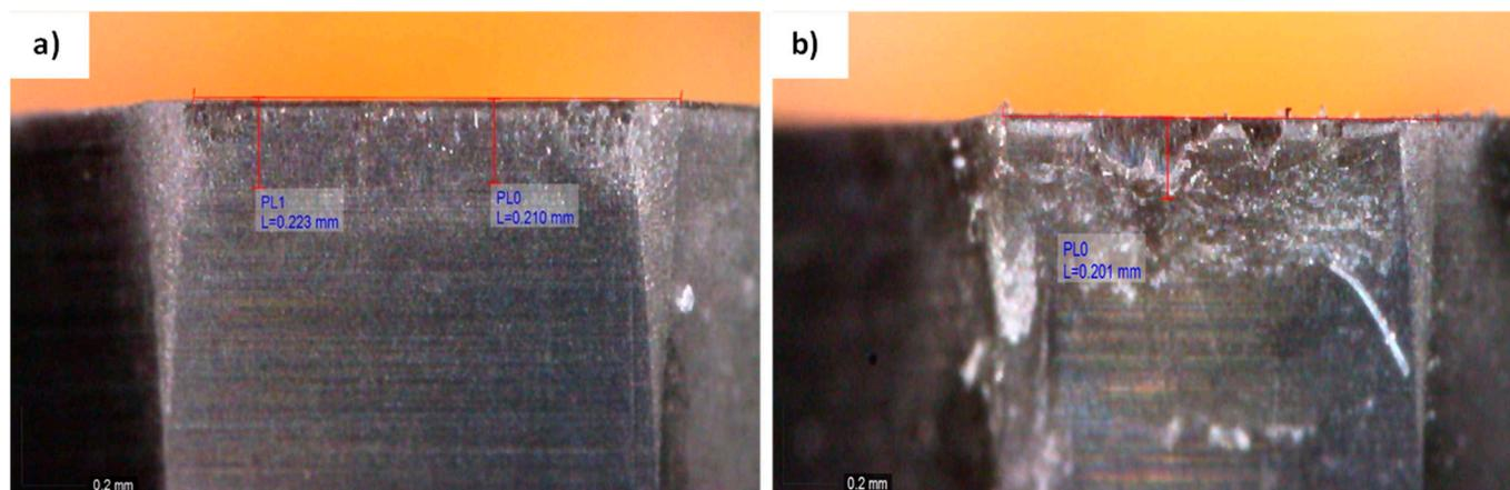
**Figure 4.** Nose region of worn tools for Experiment 7: (a): chipping or flaking and Experiment 2 (b): notching on flank face. Scale bar at 0.2 mm.
