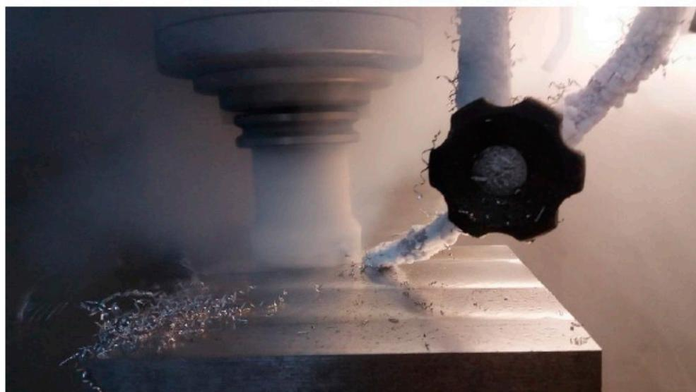
**Figure 1.** Liquid nitrogen delivery during the machining process.
