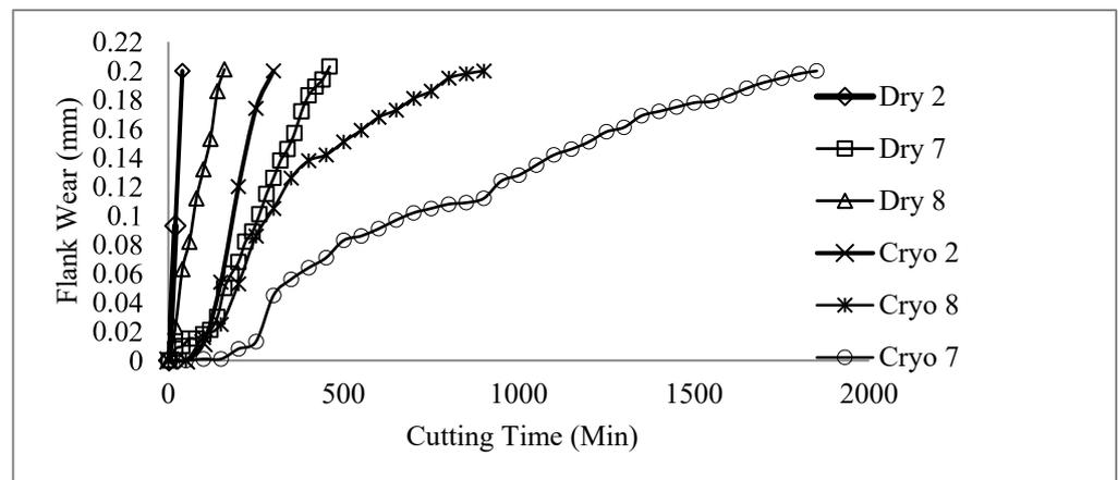
**Figure 5.** Flank wear progression for both dry and cryogenic conditions.
