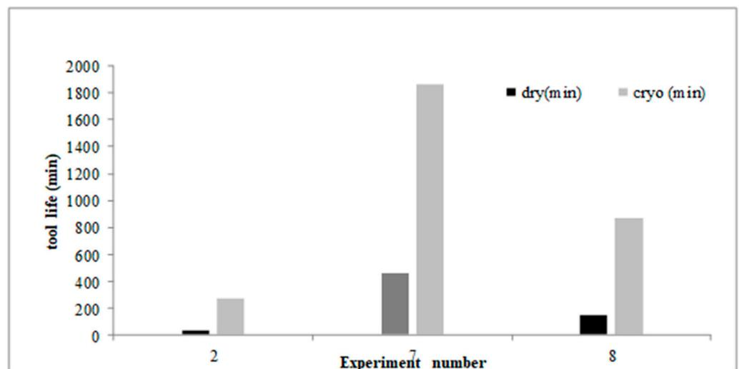
**Figure 6.** Comparison of tool life under dry and cryogenic conditions.
