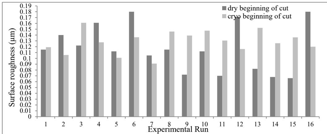
**Figure 10.** Surface roughness under dry and cryogenic conditions.
