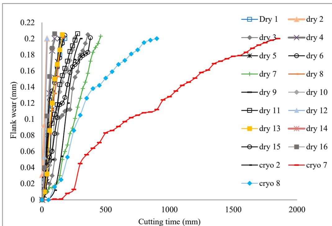
**Figure 3.** Flank wear (mm) vs. cutting time (min) for both dry and cryogenic machining based on full factorial design of study.
