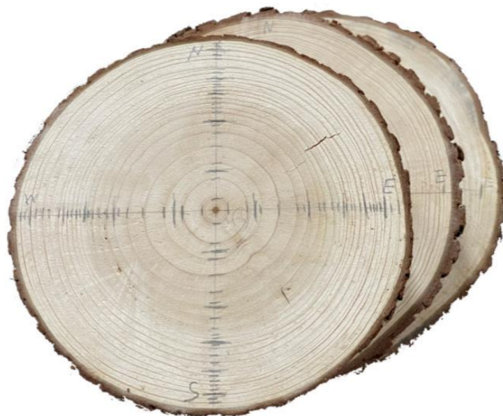
Figure 2. A representative polished disc showing the east–west and north–south diameter lines.
