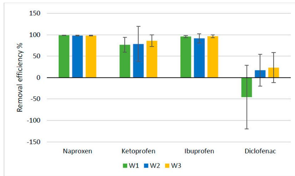
**Figure 4.** Removal efficiencies and their standard deviation bars (%) in the control and inoculated WWTPs with the preselected effective mixed bacteria culture. W1 = Ibrány as control, W2 = Levelek, W3 = Újfehértó.
