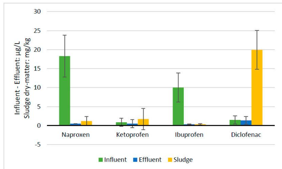
**Figure 3.** Average NSAID concentrations with standard deviation bars in pilot plant, where the target agents in the sludge content are expressed: mg/kg of the dry matter, in the influent and effluent: µg/L.
