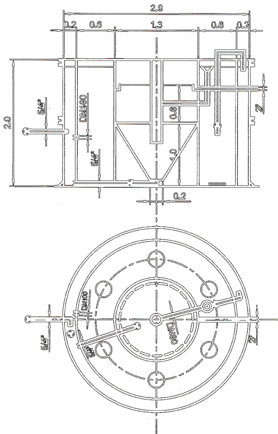
**Figure 1.** Schematic structure of the constructed experiment pilot plant; dimensions are expressed in: DN (mm); inch ("); meter (m).
