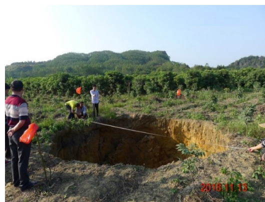
Figure 3. Sinkhole caused by mine water inflow.
