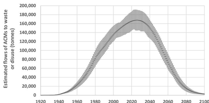
**Figure 4.** Estimated flows of asbestos containing materials to waste or disuse (tonnes).
