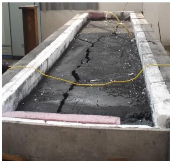
**Figure 6.** Freezing effect of cement tank overall.
