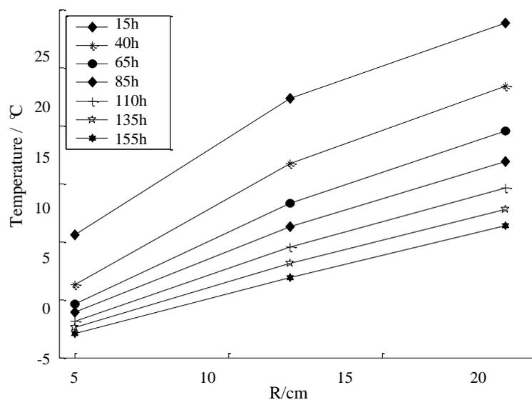
**Figure 4.** Relationship between temperature and freezing time in freezing pipe center.
