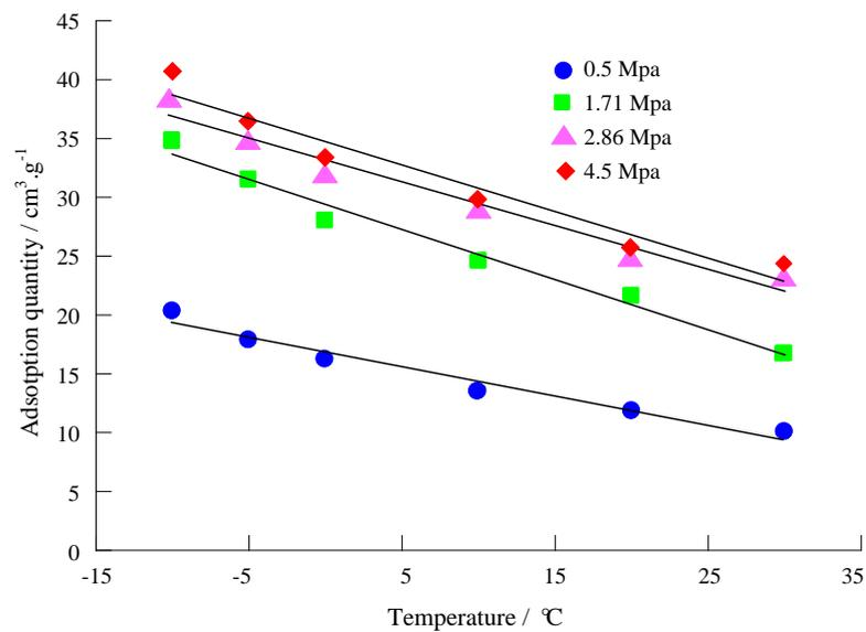
**Figure 7.** Relationship between temperature and the adsorption quantity of samples under different pressures.
