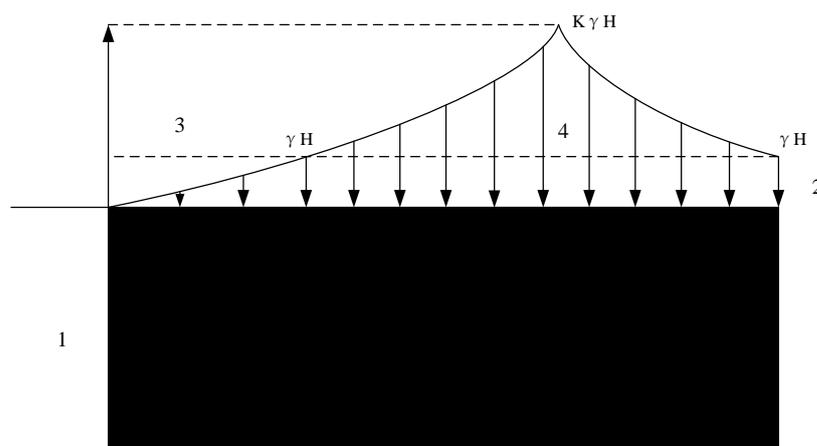
**Figure 1.** Stress distribution of coal and rock in front of roadway working face. 1—Roadway working face; 2—Original stress zone; 3—Pressure relief zone; 4—Concentrated stress zone.
