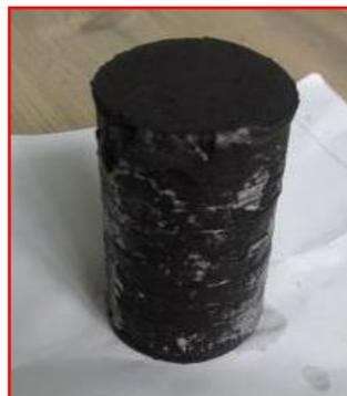
**Figure 8.** Molding coal samples from the outburst coal seam.
