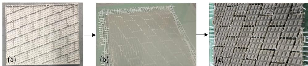
**Figure 3.** Production process of the texture layer: (a) silicone mold, (b) filling the mold and placing textile, and (c) releasing texture layer from mold.
