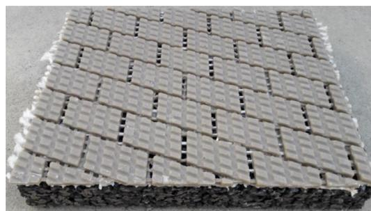
**Figure 4.** Combination of texture and absorption layer.
