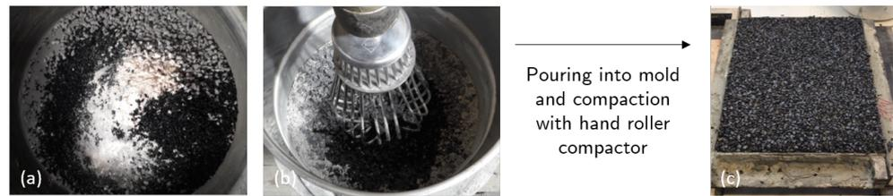
**Figure 2.** Production process of the absorption layer: (a) aggregates, (b) mixing tool, and (c) compacted mixture in mold.
