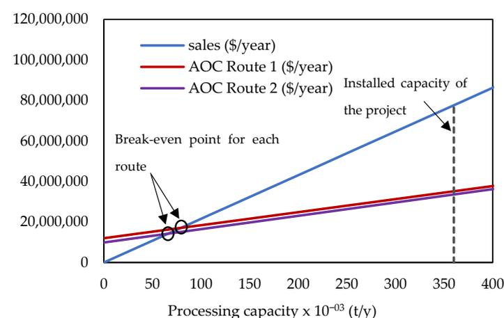
**Figure 2.** Plant resilience to hydrogen processing capacity through indirect gasification.
