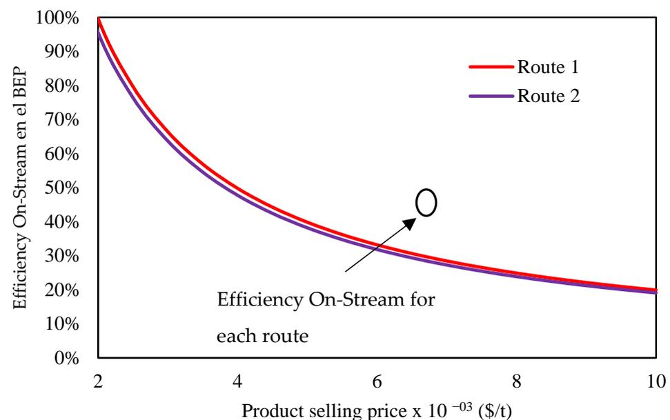
**Figure 3.** Resilience of the selling price of hydrogen production through indirect gasification with respect to on-stream efficiency at the break-even point.
