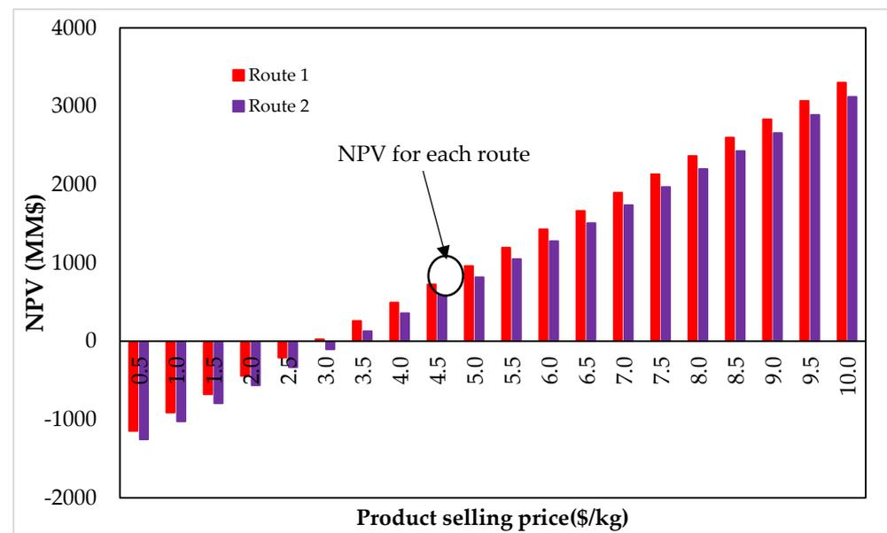
**Figure 7.** Resilience of the product selling price with respect to the normalized net present value of hydrogen production through indirect gasification.
