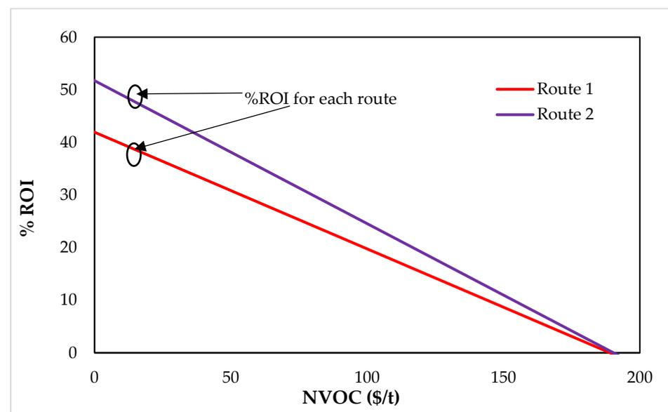
**Figure 5.** Resilience of return on investment based on the operating costs of hydrogen production through indirect gasification.
