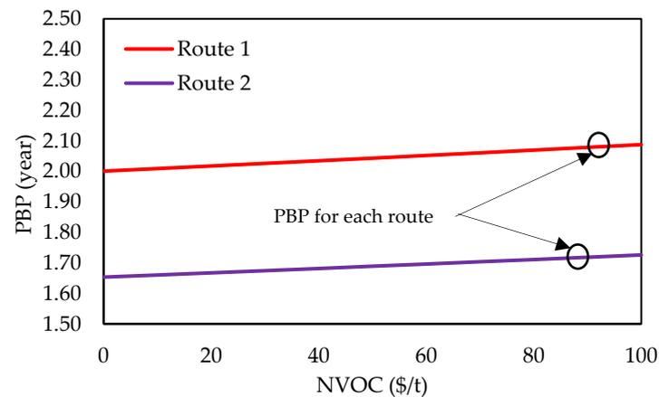
**Figure 6.** Resilience of the payback period with respect to normalized variable operating costs of hydrogen production through indirect gasification.
