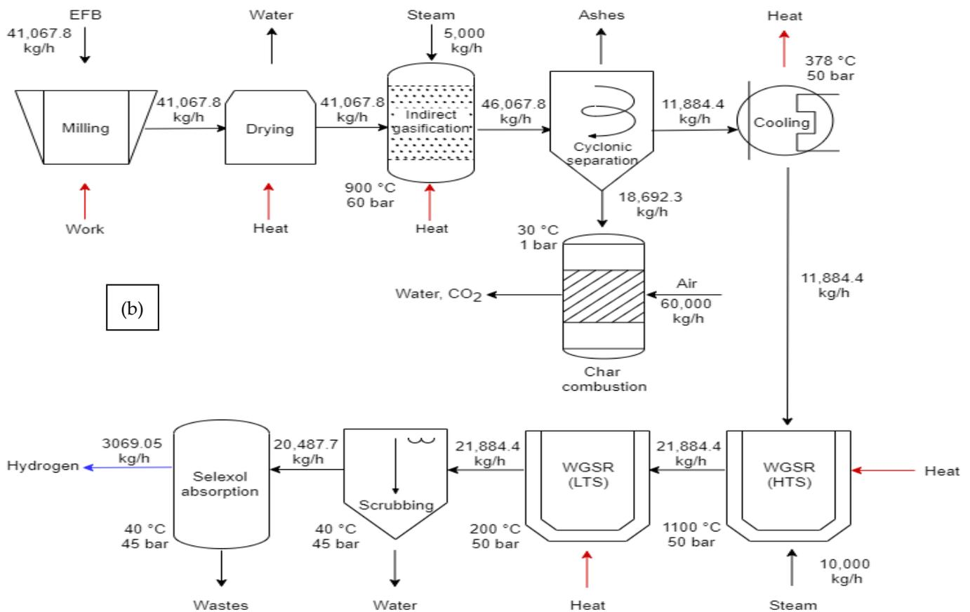
**Figure 1.** (a) Process diagram of hydrogen production by indirect gasification Route 1 (PSA); (b) Process diagram of hydrogen production by indirect gasification Route 2 (Selexol).
