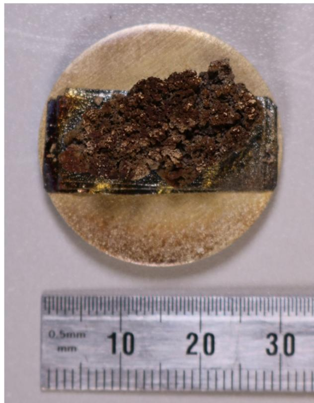
**Figure 3.** Carbon-coated sample used for the scanning electron microscopy/energy dispersive X-ray analysis.
