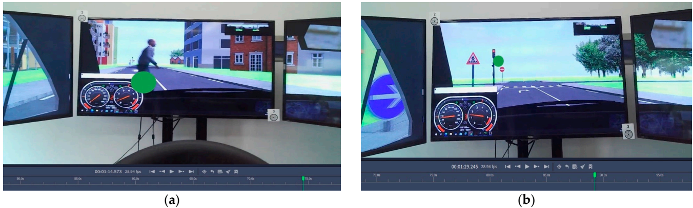
Figure 6. Pointer showing that the driver is looking at the hazard (a) and looking at the traffic signal (b) on an intersection.
