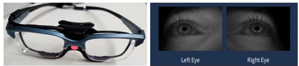
Figure 2. Asee Pro Glasses with scanned Pupils.
