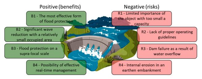
**Figure 3.** Main benefits and risks associated with the operation of reservoirs during high-water stages and flood risk.
