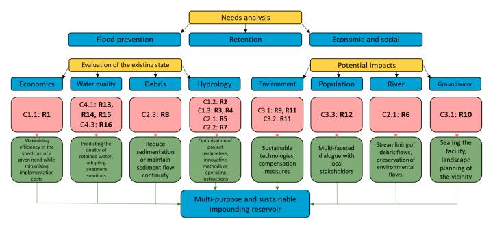
**Figure 7.** The most important issues to be considered during the planning and construction of reservoirs.
