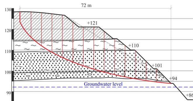
Figure 6. Calculation scheme for substantiating the III wall stability of the Pivdenno-Skhidnyi open pit.
