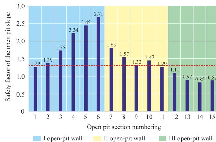
Figure 7. Safety factor for the studied open-pit wall sections (red dashed line is normative safety factor).
