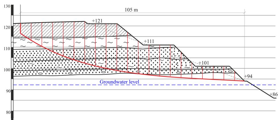
**Figure 4.** Calculation scheme for substantiating the I wall stability of the Pivdenno–Skhidnyi open pit.
