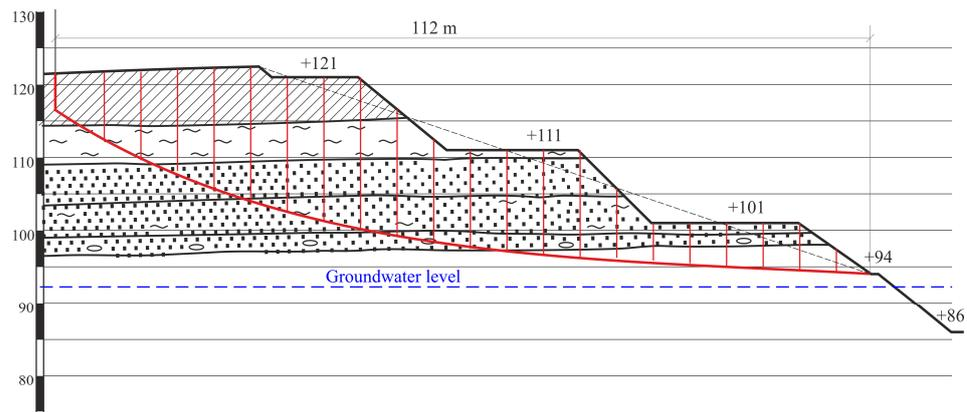
Figure 5. Calculation scheme for substantiating the II wall stability of the Pivdenno-Skhidnyi open pit.
