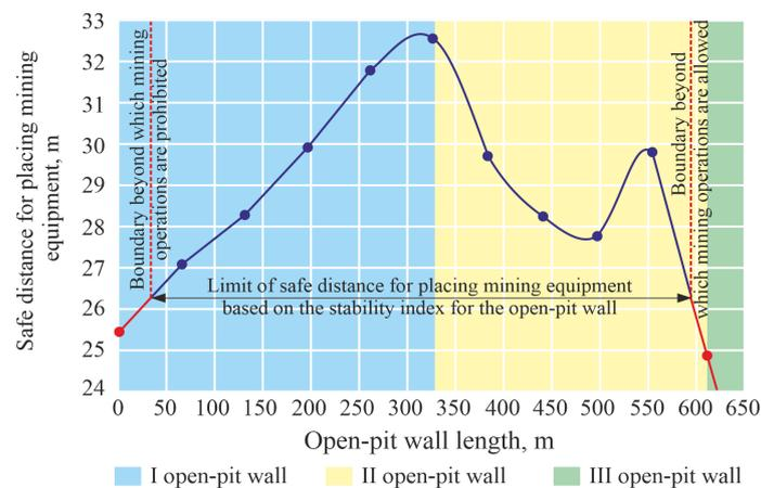
**Figure 8.** Dependence of change on the safe distance for placing mining equipment (dragline) along the strike of the open-pit walls.
