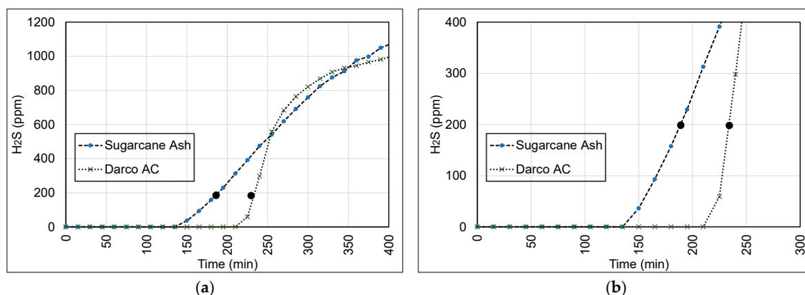
**Figure 5.** (a) H<sub>2</sub>S sorption curves for SCBA and AC. The black dots display the time corresponding to the breakthrough point for each material (Figure (b) has been augmented for better visualization of the breakthrough point).
