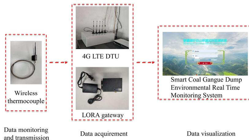
**Figure 7.** Smart dynamic cloud monitoring system.
