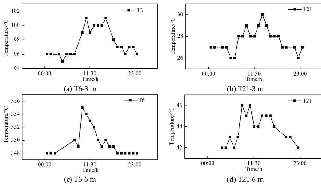
**Figure 11.** Intraday variation of coal gangue dump at different locations.
