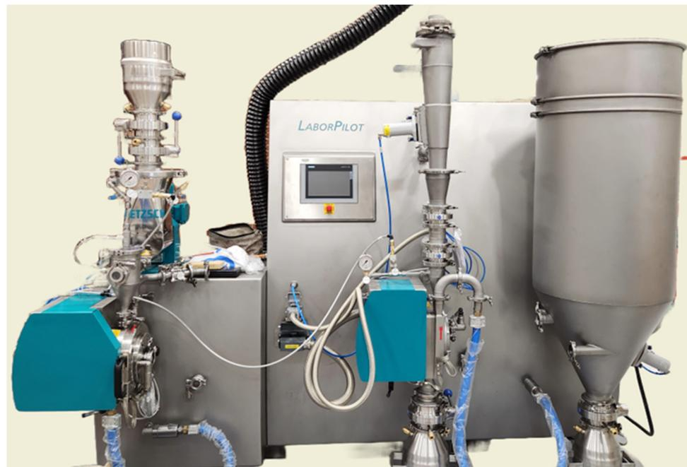
Figure 12. Image of typical jet-milling equipment.
