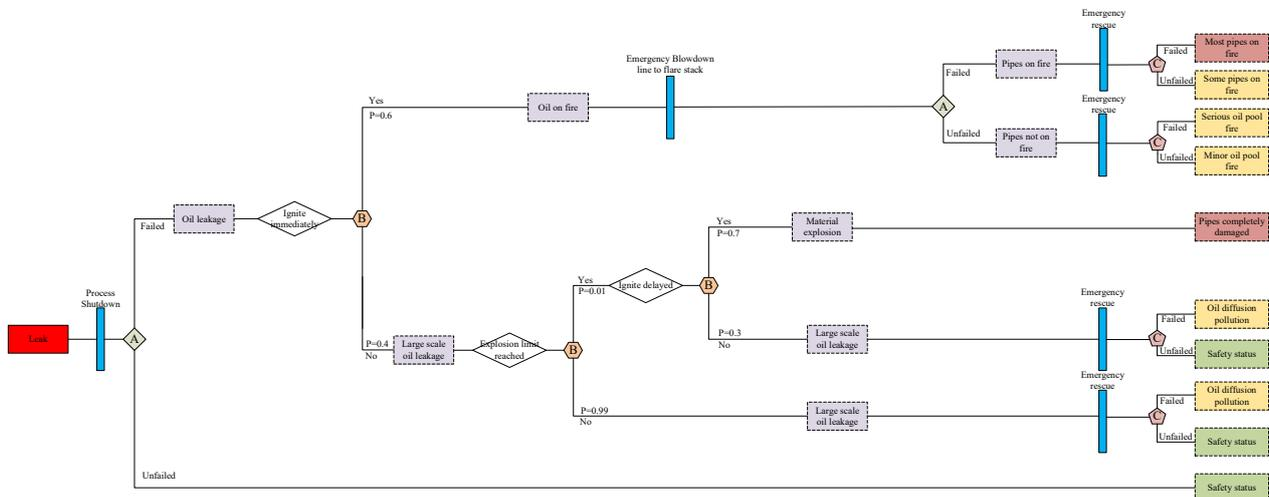
Figure 12. Event tree for pipes No.3, 7, 11, and 14.
