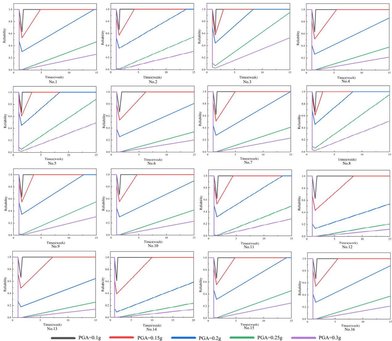
**Figure 16.** Resilience curve with reliability at different times under different PGAs.
