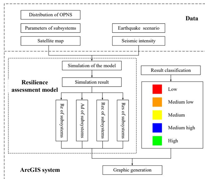
Figure 7. Framework of the OPNS resilience partitioning platform.
