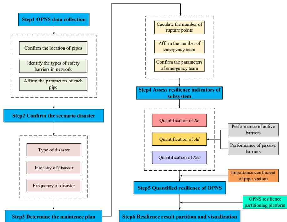
**Figure 8.** Resilience analysis methodology under an earthquake in OPNS.
