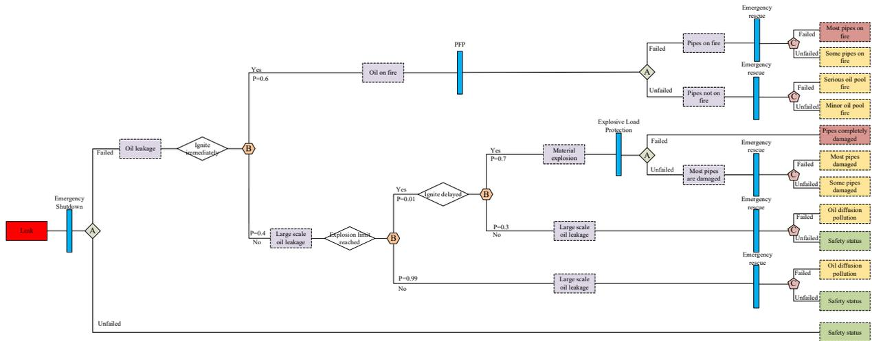
Figure 10. Event tree for pipes No.1, 4, 9, and 12.
