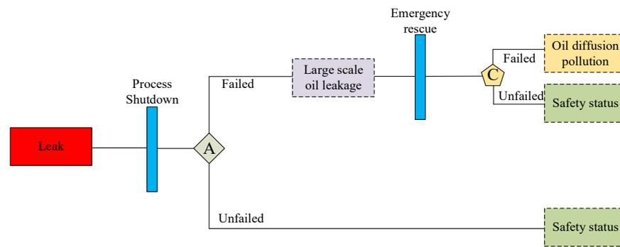
Figure 4. Event tree of pipeline system considered safety barriers.
