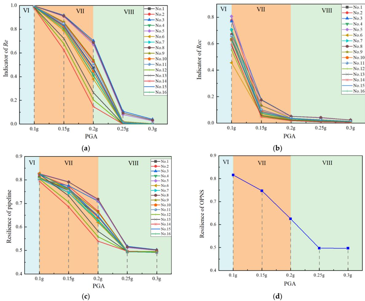
**Figure 17.** Tendency of  $Re$  and  $Rec$  under different intensities. (a) Index of  $Re$ ; (b) Index of  $Rec$ ; (c) Resilience of pipes; (d) Resilience of OPNS.
