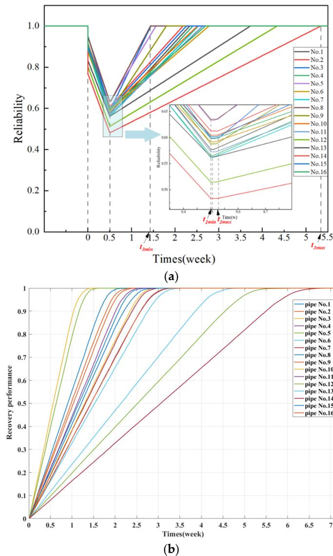
Figure 14. Resilience curve and recovery performance curve of OPNS. (a) Resilience curve with reliability at different times; (b) Recovery performance curve of pipes in OPNS.
