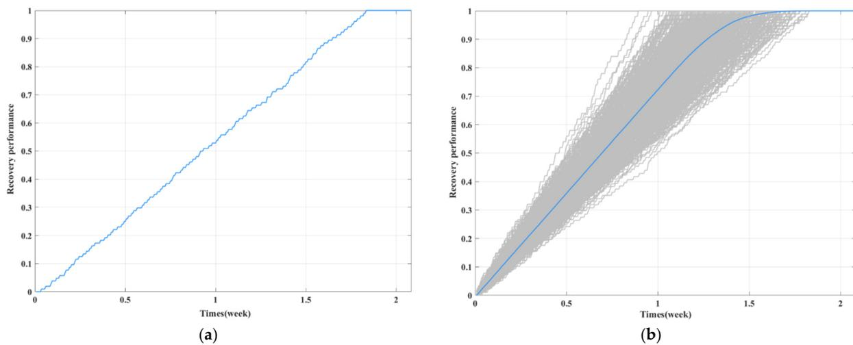
Figure 6. Recovery performance curve of pipeline. (a) single iteration; (b) 5000 iterations.
