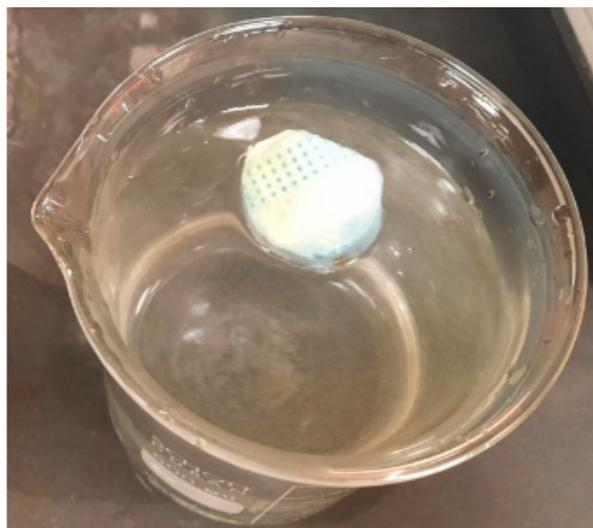
**Figure 5.** The beaker and the composite specimen used for the swelling test.
