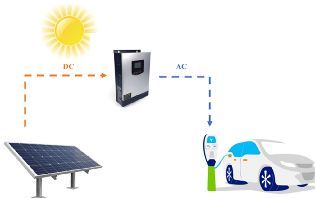
Figure 14. Schematic of a solar charger for EVs.
