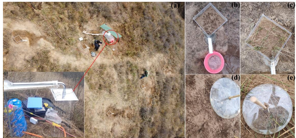
Figure 4. Simulated rainfall experiment: (a) test scenario and equipment; (b) bare soil plot after simulated rainfall; (c) grass plot after simulated rainfall; (d) details of bare soil plot after simulated rainfall; (e) details of grass plot after simulated rainfall.
