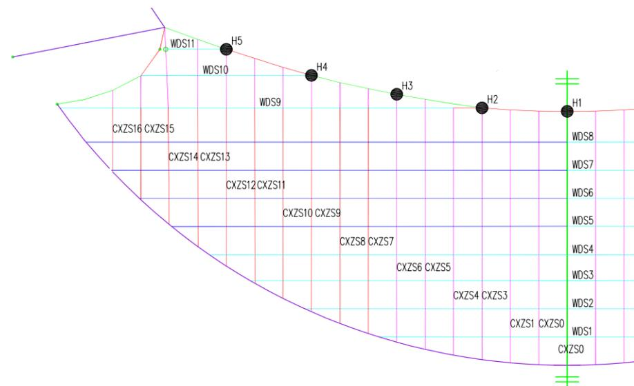
Figure 12. Cable network numbering diagram.
