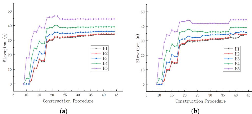
**Figure 15.** Development history of the elevation of the ring cable clamp during the entire construction process: (a) finite element simulation analysis results; (b) monitoring data of onsite construction process.
