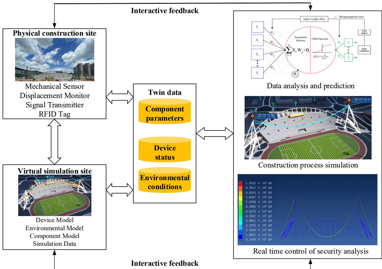
Figure 3. Digital twin framework for the construction process of cable net structure.
