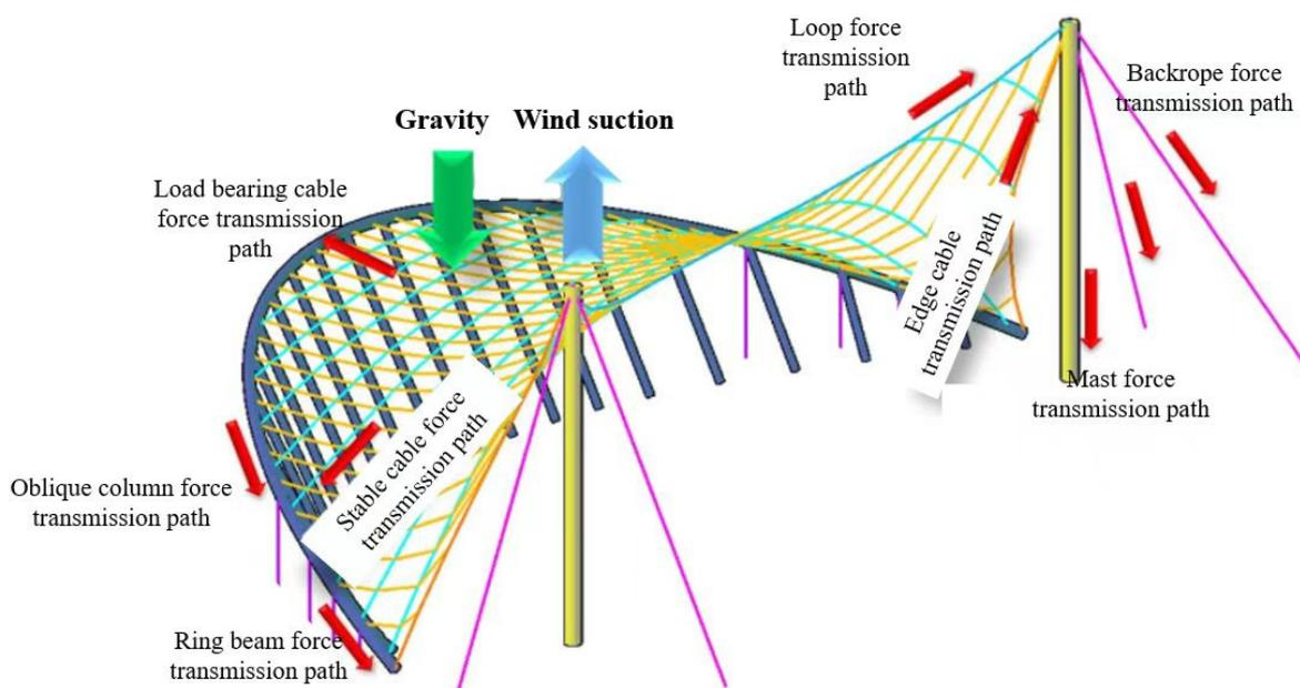
**Figure 8.** Cable structure force transmission path.
