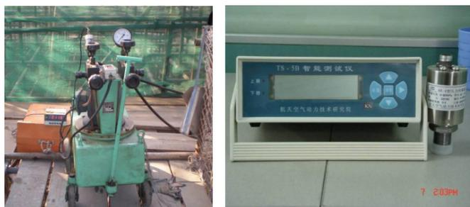
**Figure 9.** The oil pump and supporting oil pressure sensor.
