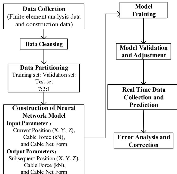
**Figure 6.** Flowchart of prediction algorithm.
