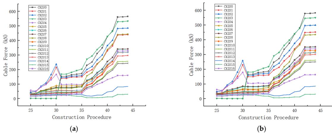
Figure 13. Development process of load-bearing cable (ring cable side) cable force during the entire construction process: (a) finite element simulation analysis results; (b) monitoring data of onsite construction process.
