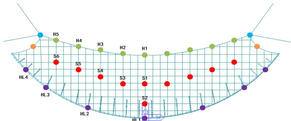
**Figure 11.** Layout of measurement points.
