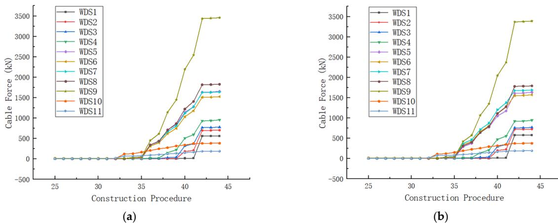
Figure 14. Development history of stable cable force throughout the construction process: (a) finite element simulation analysis results; (b) monitoring data of onsite construction process.
