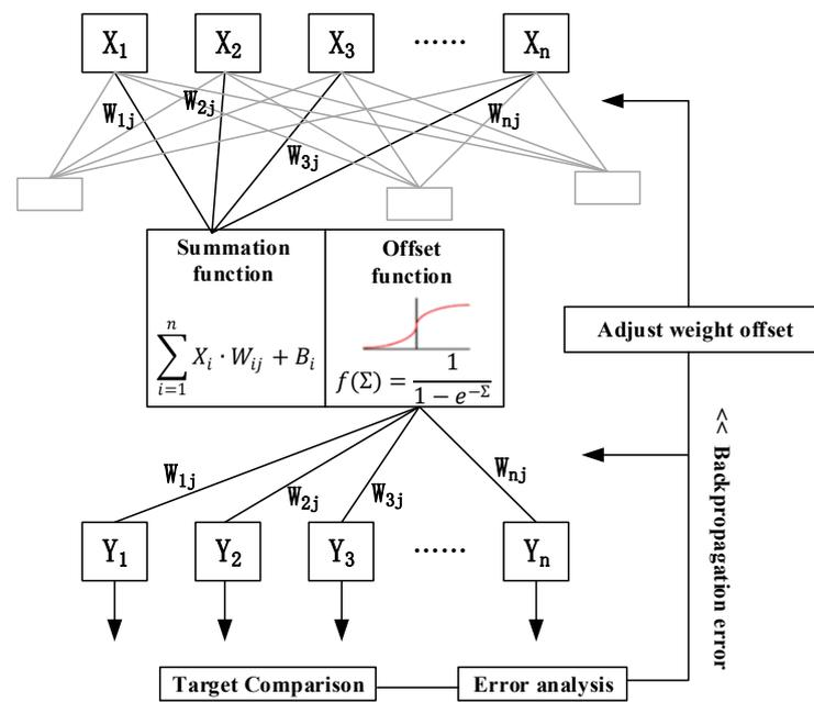
**Figure 5.** Structure and mathematical representation of BP artificial neurons (hidden neurons).
