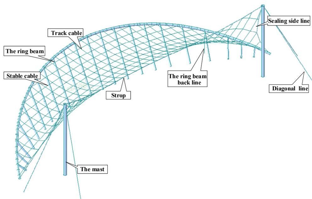
Figure 7. Three-dimensional structure diagram.
