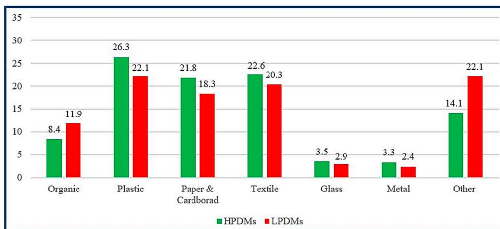
**Figure 7.** Waste fractions of HPDMs and LPDMs (%).
