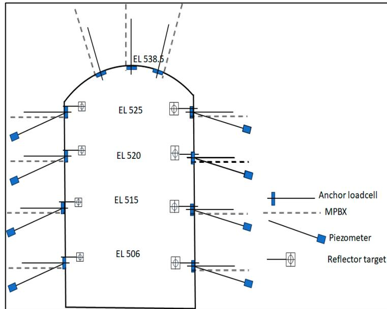
Figure 3. Typical instrumentation layout of an underground cavern.
