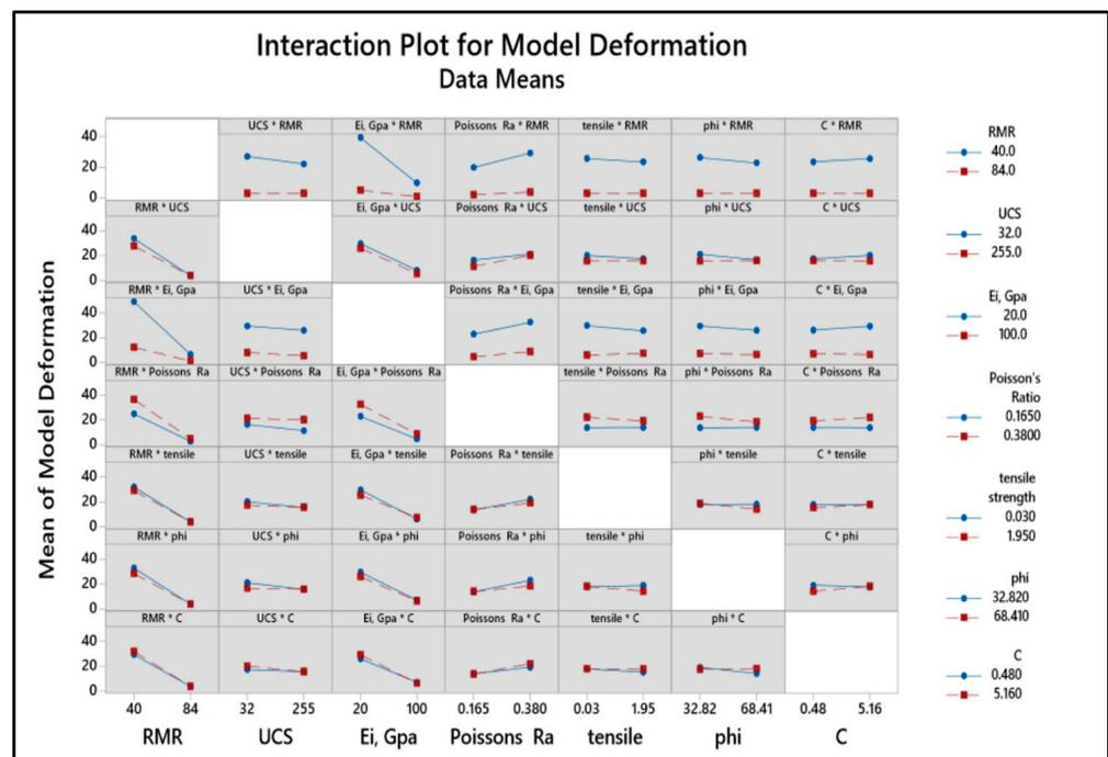
Figure 10. Interaction effects plot of crown deformation between different variables of MHP-MH cavern.
