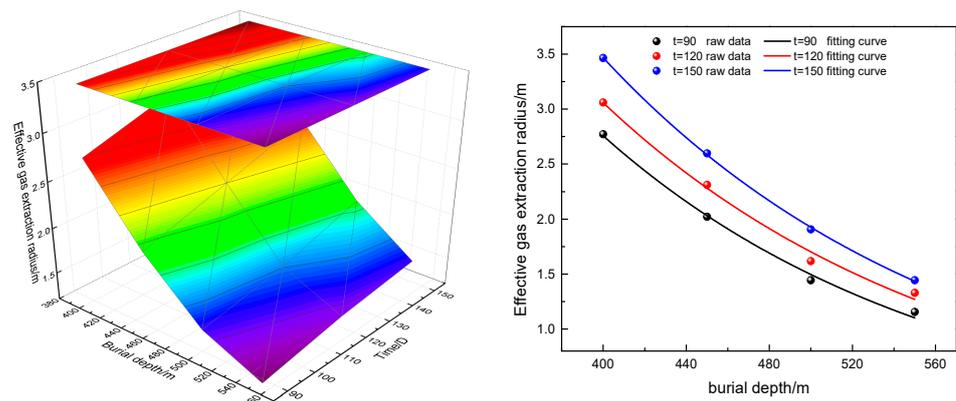
**Figure 17.** The fitted curve between the gas extraction radius and the burial depth.
