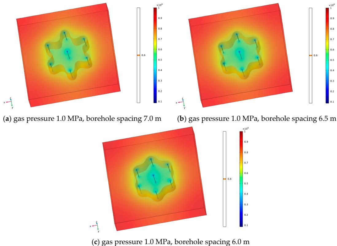
**Figure 10.** The gas isobaric surface shape at different gas pressure ( $t = 120$  D).
