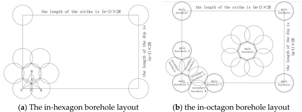
Figure 2. The in-hexagon and the in-octagon borehole layout.
