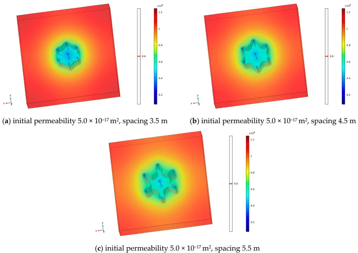
**Figure 13.** The gas isobaric surface shape at different initial permeabilities ( $T = 120 \text{ D}$ ).
