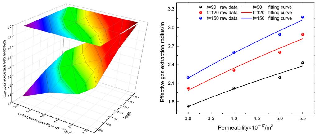
**Figure 14.** The fitted curve between the gas extraction radius and the initial permeability.
