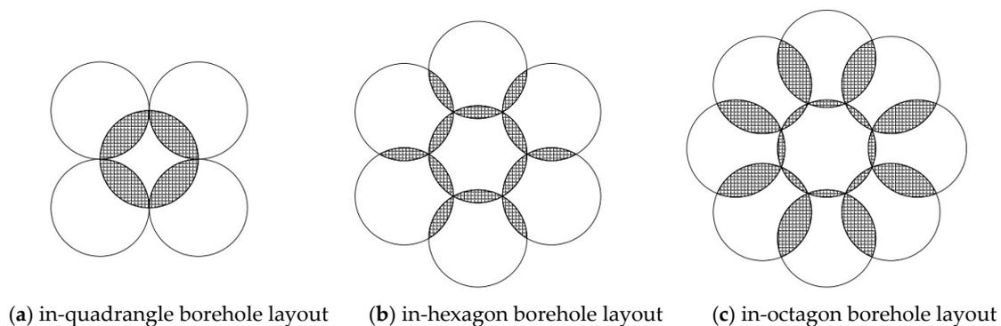
**Figure 3.** The extraction redundant area of in-polygon borehole layout.
