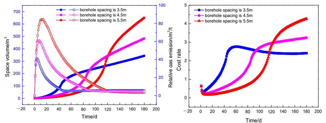
Figure 12. The evolution of extraction parameters with time for initial permeability ( $5.0 \times 10^{-17} \text{ m}^2$ ).
