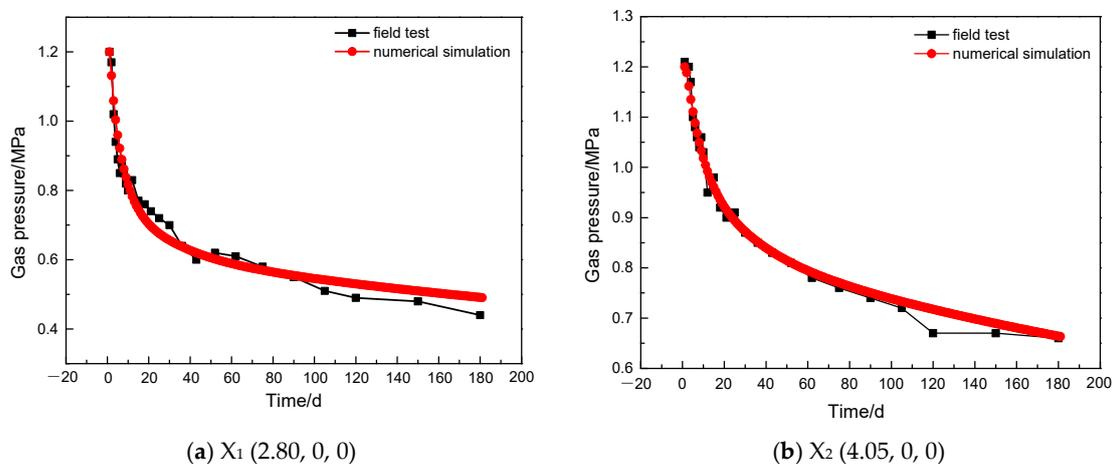
Figure 7. The curves of gas pressure from numerical simulations and field tests.
