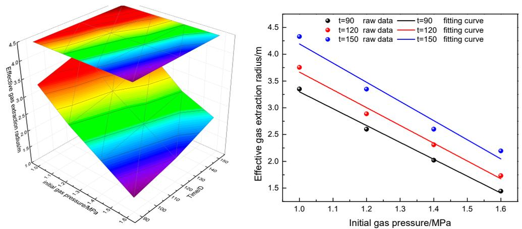
Figure 11. The fitted curve between the gas extraction radius and the initial gas pressure.
