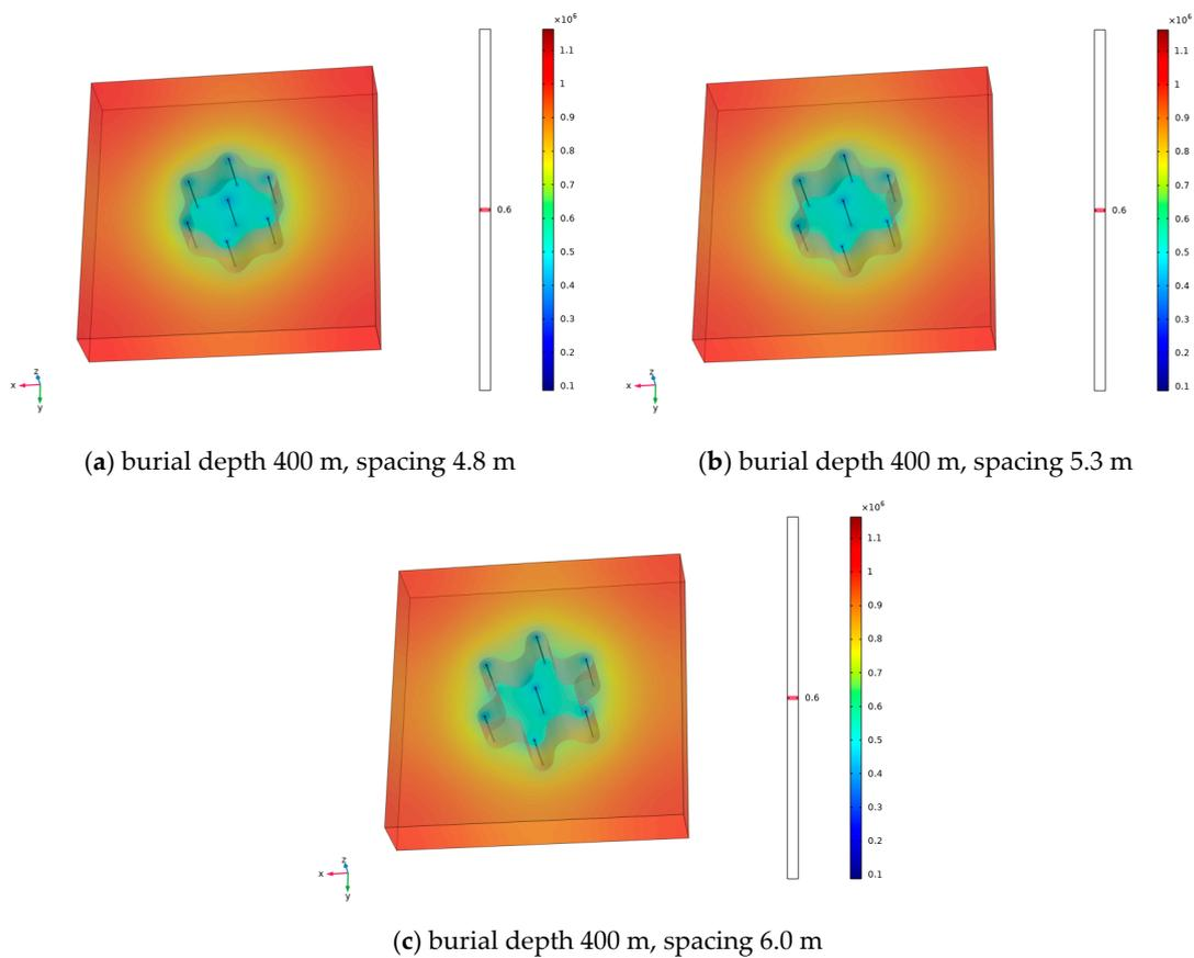
Figure 16. The gas isobaric surface shape at different buried depths ( $t = 120$  D).
