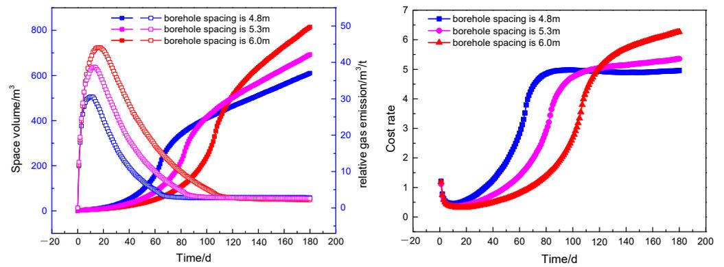
Figure 15. The evolution of extraction parameters with time for burial depth (400 m).
