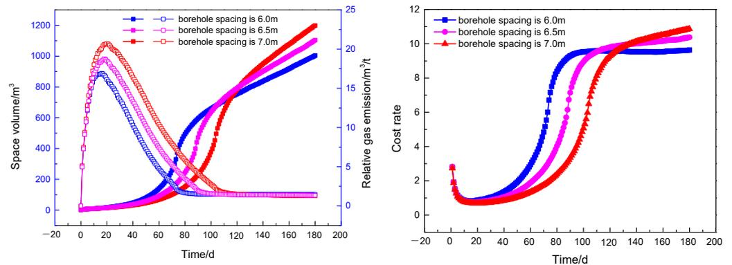
**Figure 9.** The evolution of extraction parameters with time for initial gas pressures (1.0 MPa).
