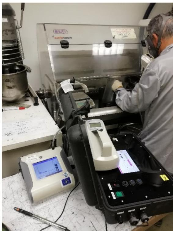
**Figure 13.** Setup developed to perform the particulate matter exposition campaign at the industrial facility.
