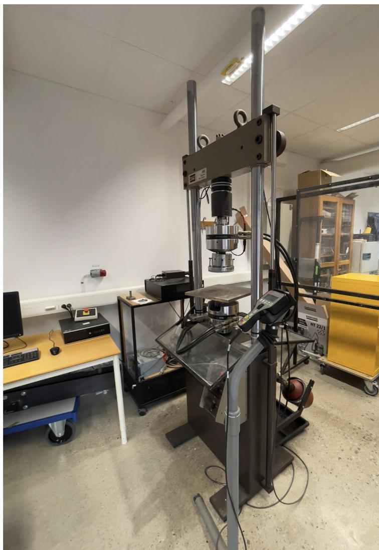
**Figure 7.** MTS 810 servohydraulic universal testing machine with maximum force capacity of 10 t in compression/tension used for test compressive strength of the specimens. Photo: Per Lindh.
