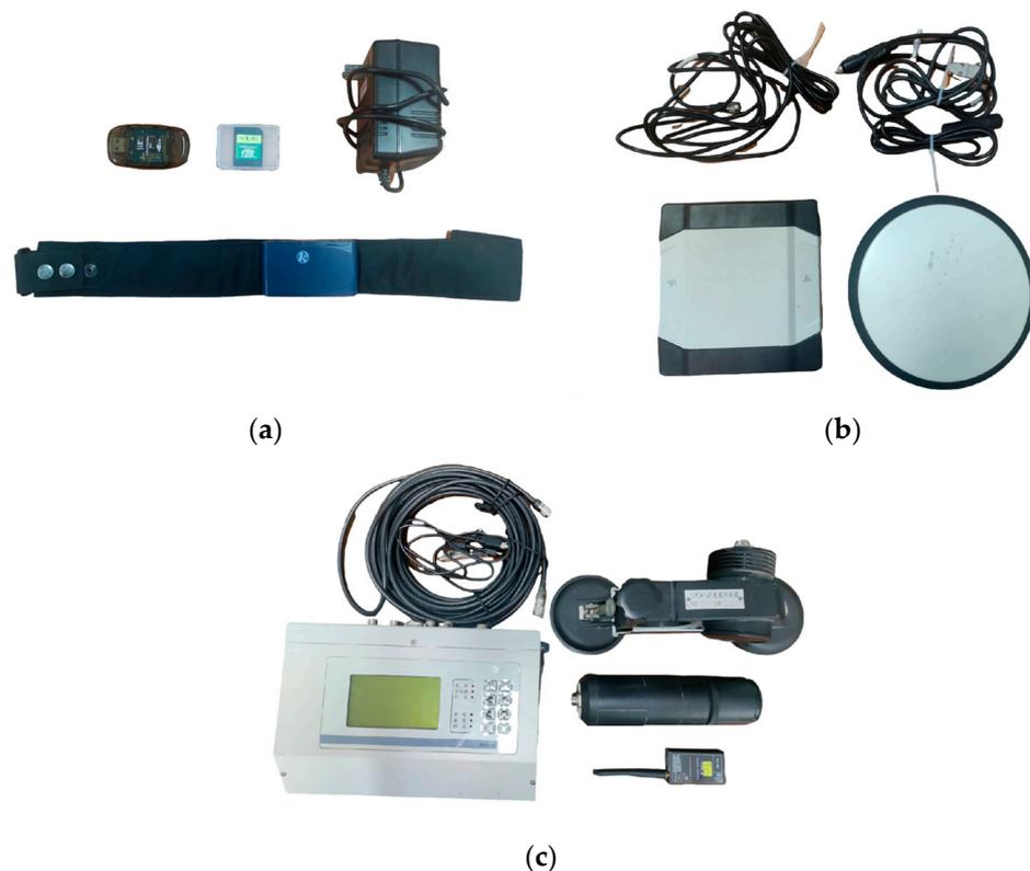
**Figure 1.** Instruments and equipment used in the experiment. (a) Physiological detector; (b) Dynamic GPS; (c) non-contact multifunctional speedometer.
