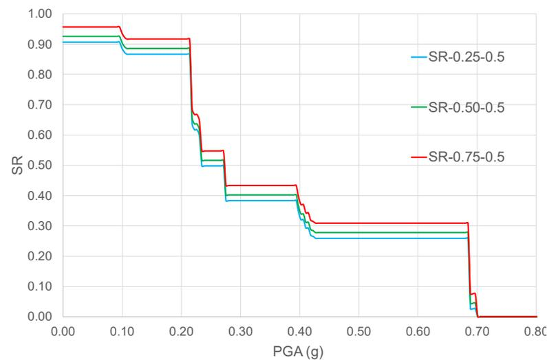
**Figure 8.** PGA (g) Vs SR ( $c = 0.5$  and  $r/r_0 = 0.25, 0.50, 0.75$ ).
