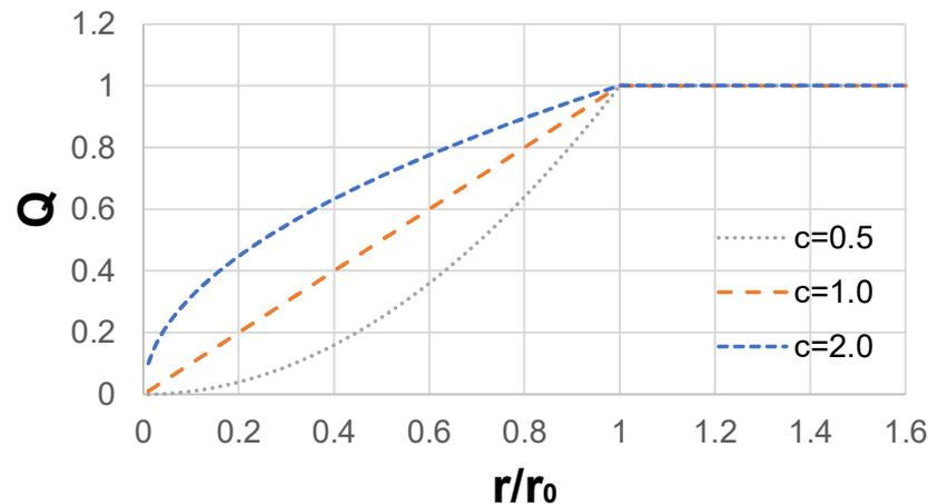
**Figure 2.** Definition of redundancy ( $r$ ) based on Equation (2).
