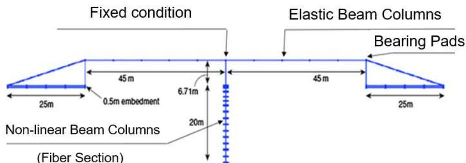
**Figure 6.** Numerical model of Bridge B1 (vertical view).
