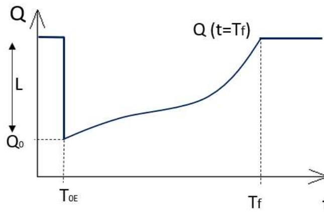
**Figure 1.** Definition of Seismic Resilience ( $SR$ ,  $t$  = time,  $L$  = losses;  $T_f$  = time of finishing the repair work;  $Q$  = functionality;  $T_{OE}$  = time of occurrence of the earthquake).
