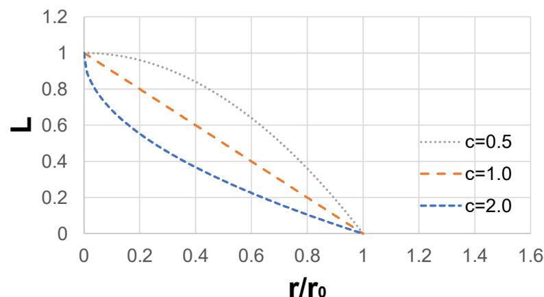
**Figure 3.** Definition of losses ( $L$ ) based on Equation (2).
