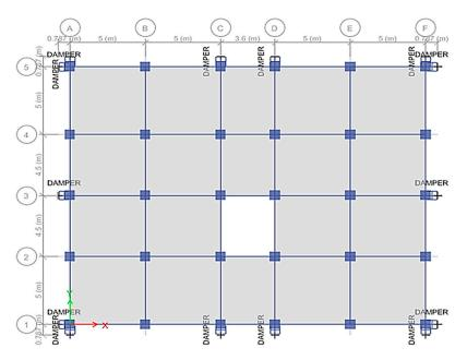
Figure 9. Plan view of damper placement on upper basement.
