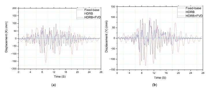
**Figure 18.** Displacement comparison for the three models (fixed-base, HDRB isolated, HDRB+FVD isolated) in Dar El-Beïda; (a) in the X direction; (b) in the Y direction.
