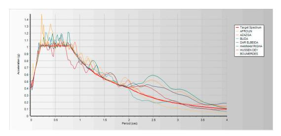
Figure 12. Code-conforming spectrum-compatibility check of the selected records according to EC8.
