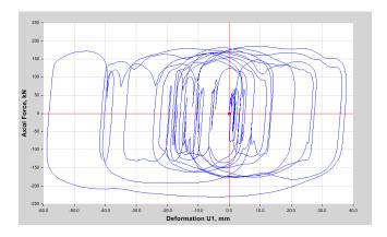
Figure 14. FVD's hysteresis loops (data from Dar El Beïda seismic record).
