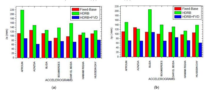
**Figure 19.** Displacement comparison for the three models (fixed-base, HDRB isolated, HDRB+FVD isolated) for different accelerograms; (a) in the X direction; (b) in the Y direction.
