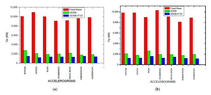
**Figure 16.** Base shear comparison for the three models (fixed-base, HDRB isolated, HDRB+FVD isolated) for different accelerograms; (**a**) in the X direction; (**b**) in the Y direction.
