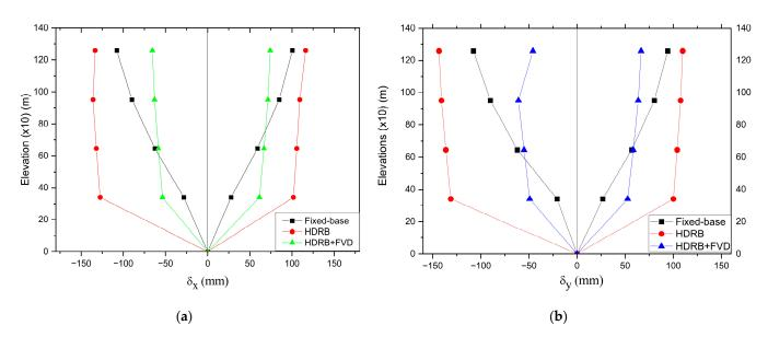
Figure 20. Average displacement for different levels; (a) in the X direction; (b) in the Y direction.
