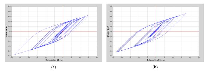
**Figure 13.** HDRB's hysteresis area (data from Dar El Beïda seismic record): (a) in the X direction; (b) in the Y direction.
