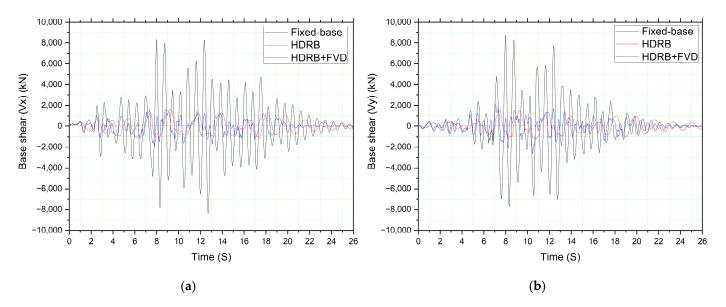
**Figure 15.** Base shear comparison for the three models (fixed-base, HDRB isolated, HDRB+FVD isolated) in Dar El-Beïda; (a) in the X direction; (b) in the Y direction.
