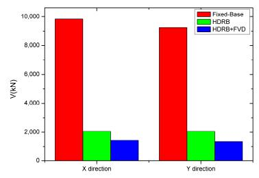
**Figure 17.** Average of base shear forces in the X and Y directions.
