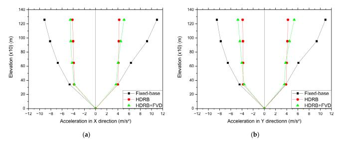
**Figure 24.** Acceleration comparison for the three models (fixed-base, HDRB isolated, HDRB+FVD isolated) for different levels; (a) in the X direction; (b) in the Y direction.
