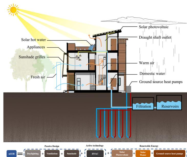
Figure 1. Diagram of the case building.
