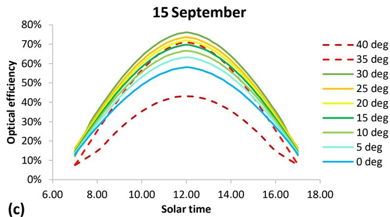
Figure 8. Daily optical efficiency results: (a) 16 March, (b) 11 June, and (c) 15 September.
