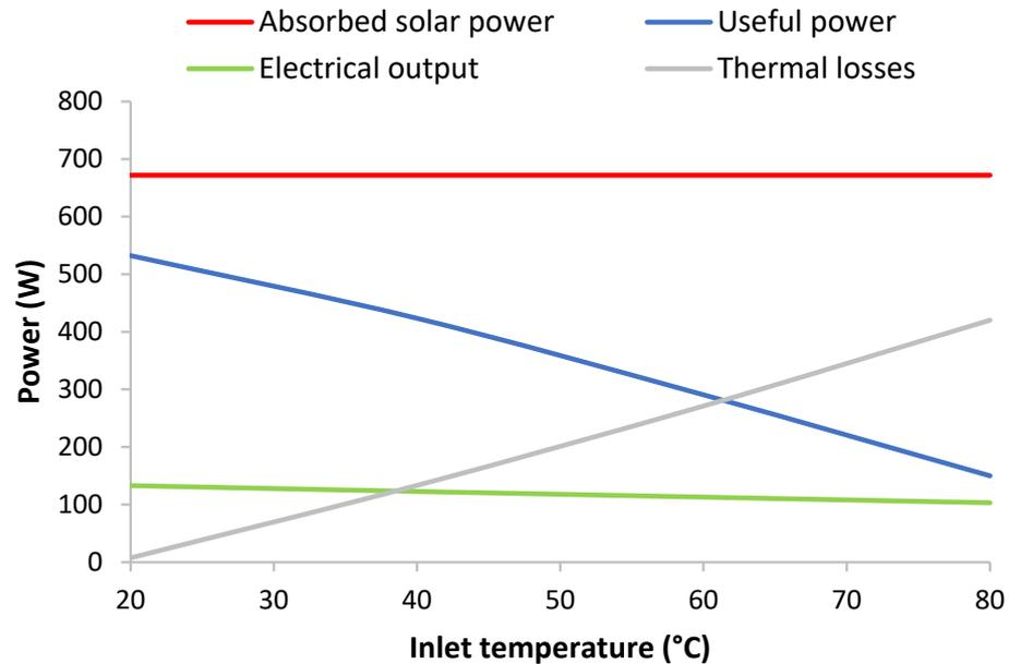
**Figure 11.** Absorbed solar power, Useful power, Thermal losses, and Electrical output of the collector in the whole inlet temperature range.
