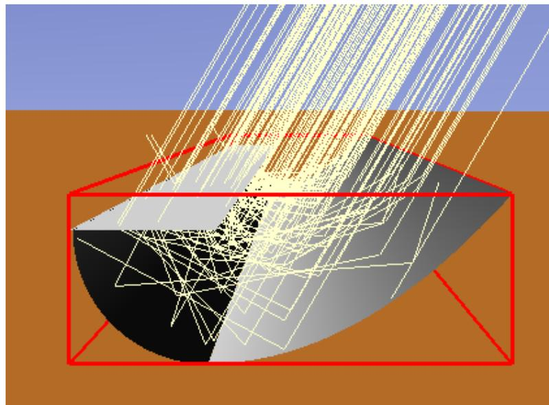
Figure 6. Ray-tracing modeling of the collector in Tonatiuh.
