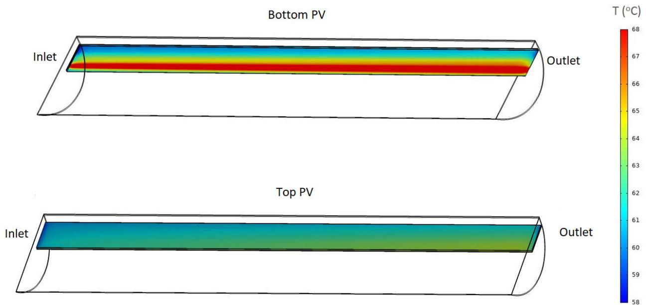
**Figure 13.** Temperature allocations of the top and the bottom PV of the receiver for  $T_{f,i} = 60$  °C.
