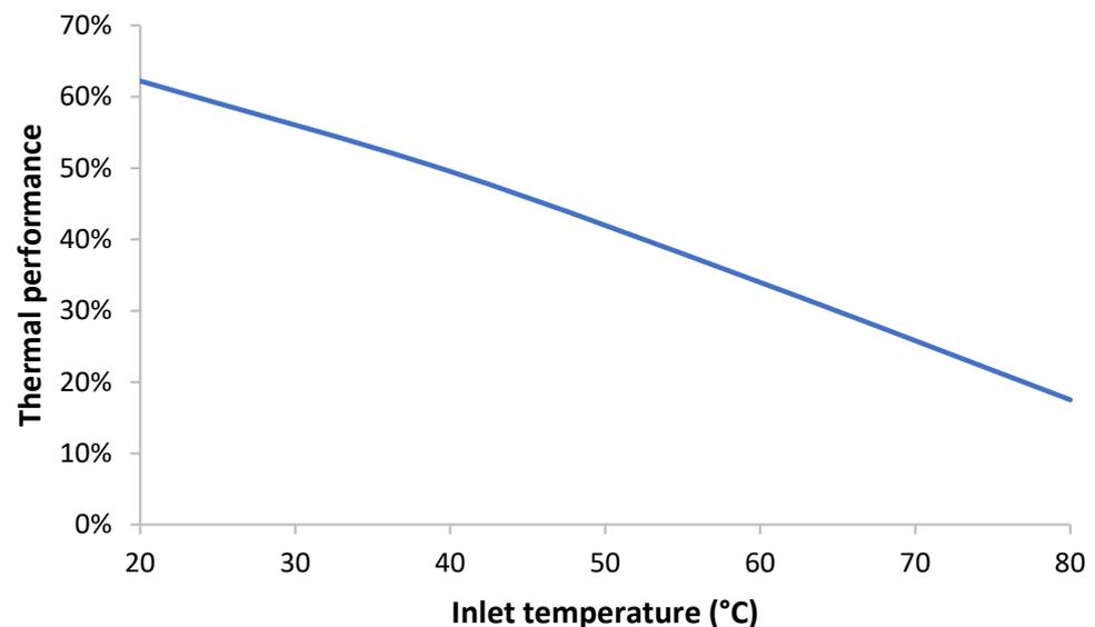
Figure 10. Thermal efficiency of the collector in the entire inlet temperature range.
