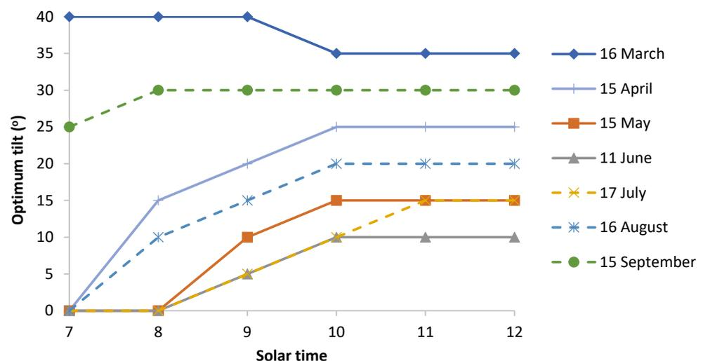
Figure 9. Optimum tilt of the collector for each operating hour of each mean day.
