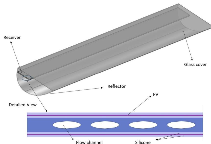
**Figure 1.** Three-dimensional (3D) collector's geometry and detailed view of the receiver.
