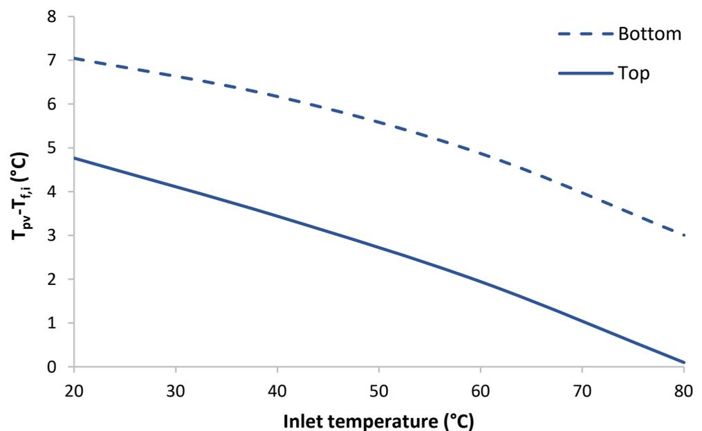
**Figure 12.** Temperature difference of the bottom and the top PV with the inlet water.
