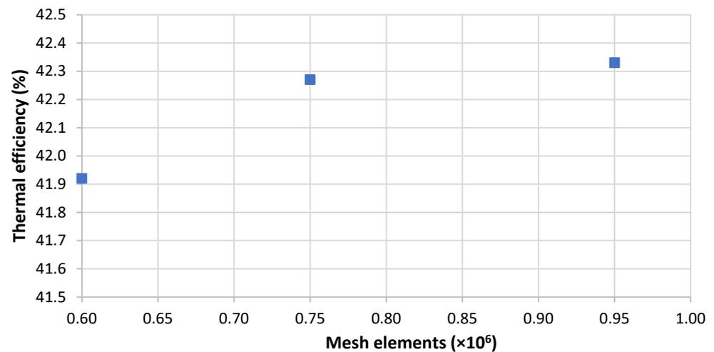
**Figure 3.** Mesh independency of the numerical model in COMSOL.
