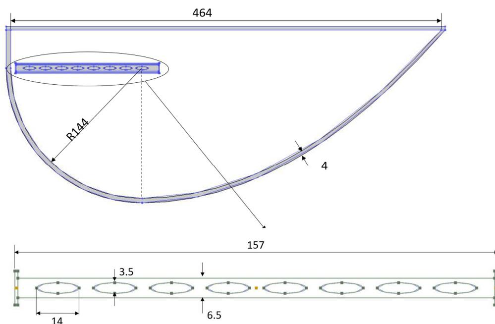
**Figure 2.** Main dimensions of the solar collector.
