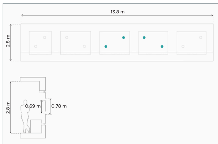
Figure 2. Elevation plan and section plan of the west wall in the test room. The openings opened for natural ventilation in this study are highlighted in blue.
