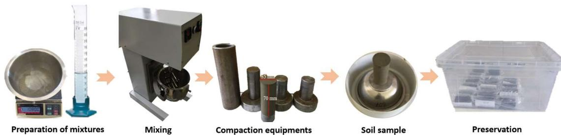
Figure 3. Sample preparation process.
