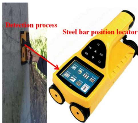
Figure 17. Steel bar position detection.
