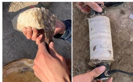
**Figure 14.** Field block wave velocity test diagram.
