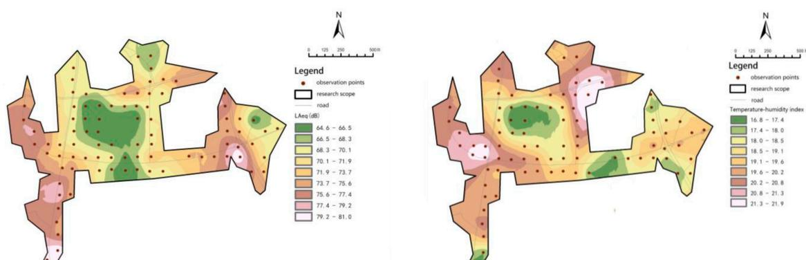
**Figure 3.** Spatial distribution of  $L_{Aeq}$  (left) and temperature–humidity index (right).
