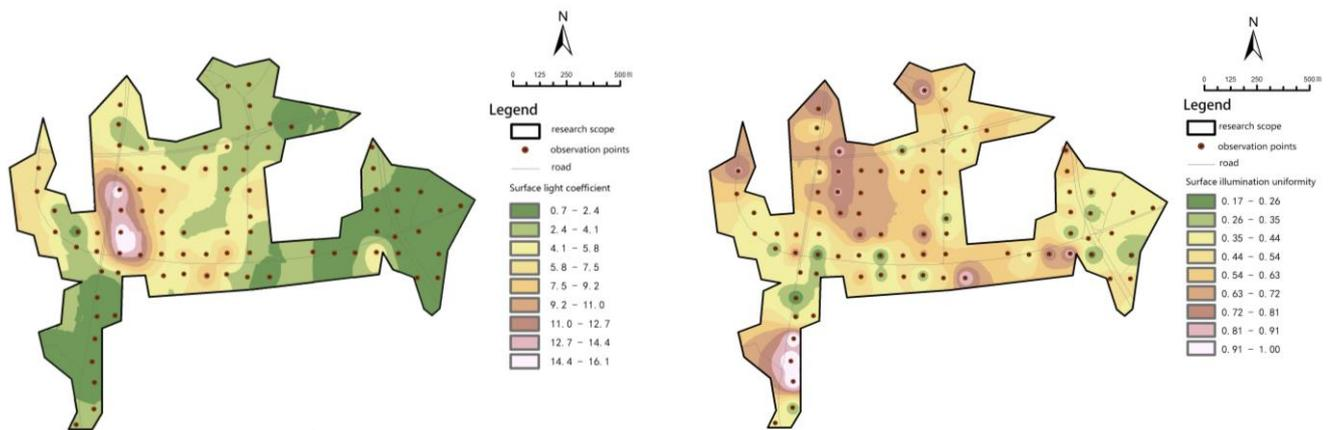
**Figure 4.** Spatial distribution diagram of surface light coefficient in outdoor space (left) and surface illumination uniformity (right).
