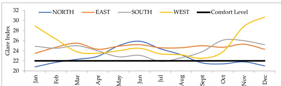
**Figure 5.** Calculated glare index value at various orientations of the office building model.
