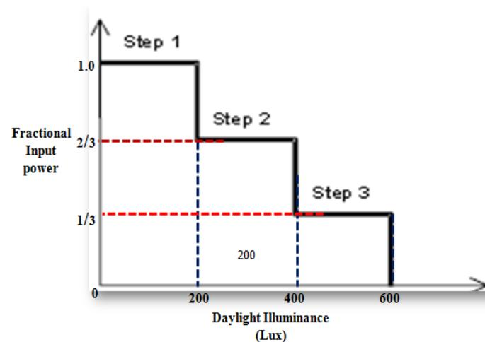
**Figure 3.** Stepped lighting control mechanism with different illumination levels.
