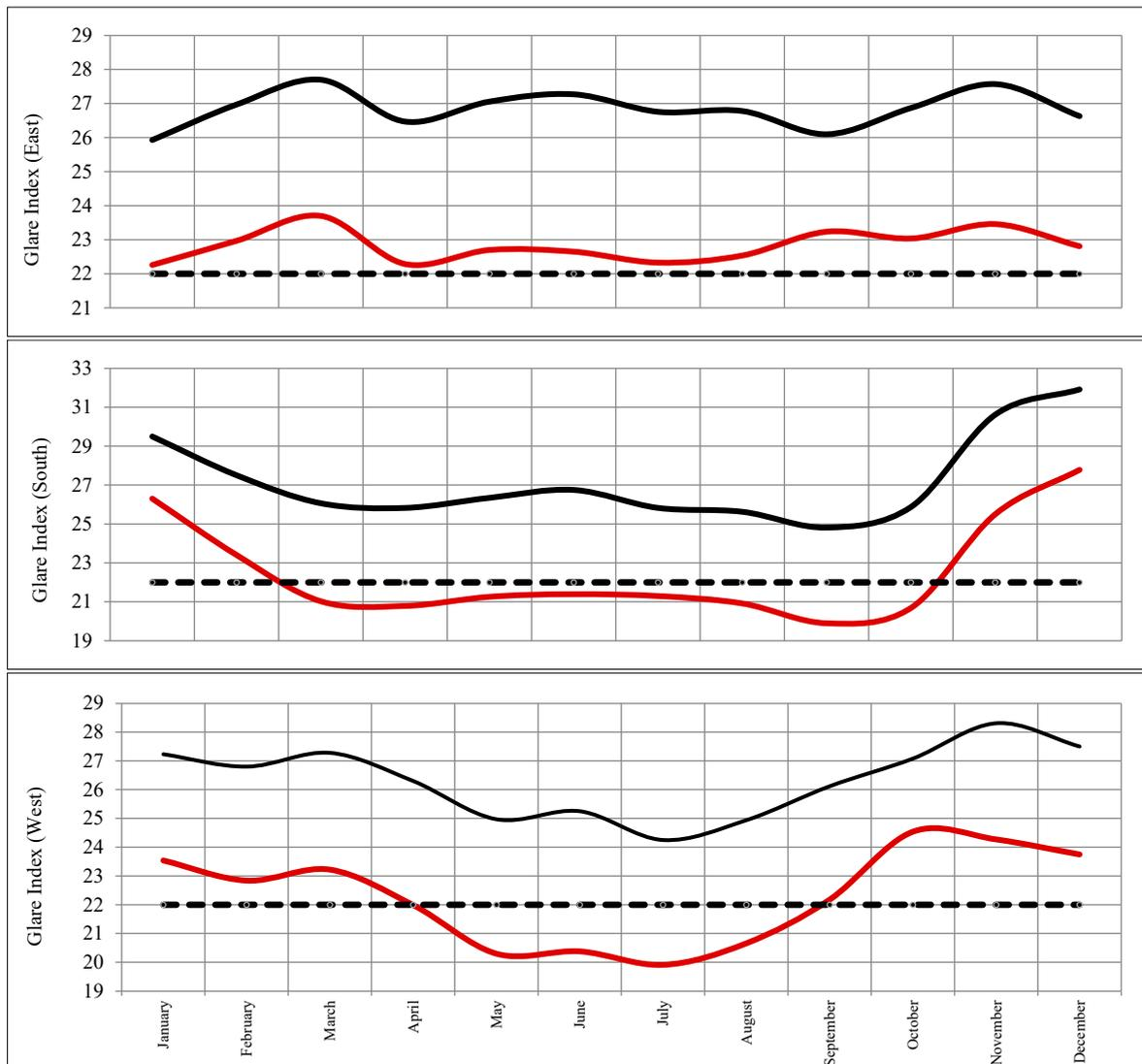
**Figure 6.** Variation in the maximum glare index value for the modeled office building with low-E and EC smart glass windows with daylight controllers at different orientations.
