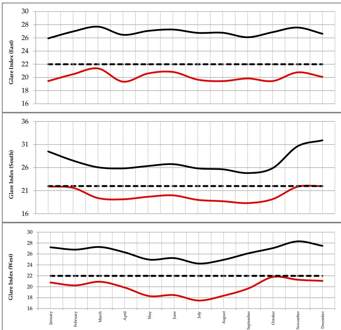
**Figure 7.** Variation in the maximum glare index value for the modeled office building with low-E and electrochromic smart glass windows with glare controller.
