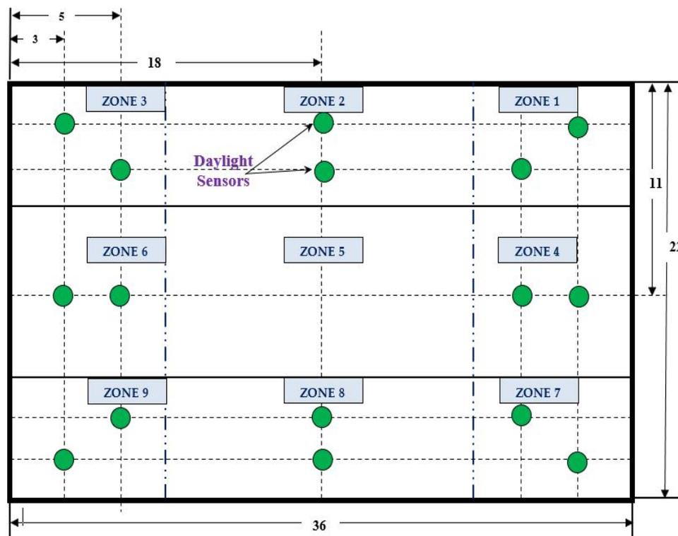
Figure 1. Office building base case plan with location of daylight sensors for different zones.
