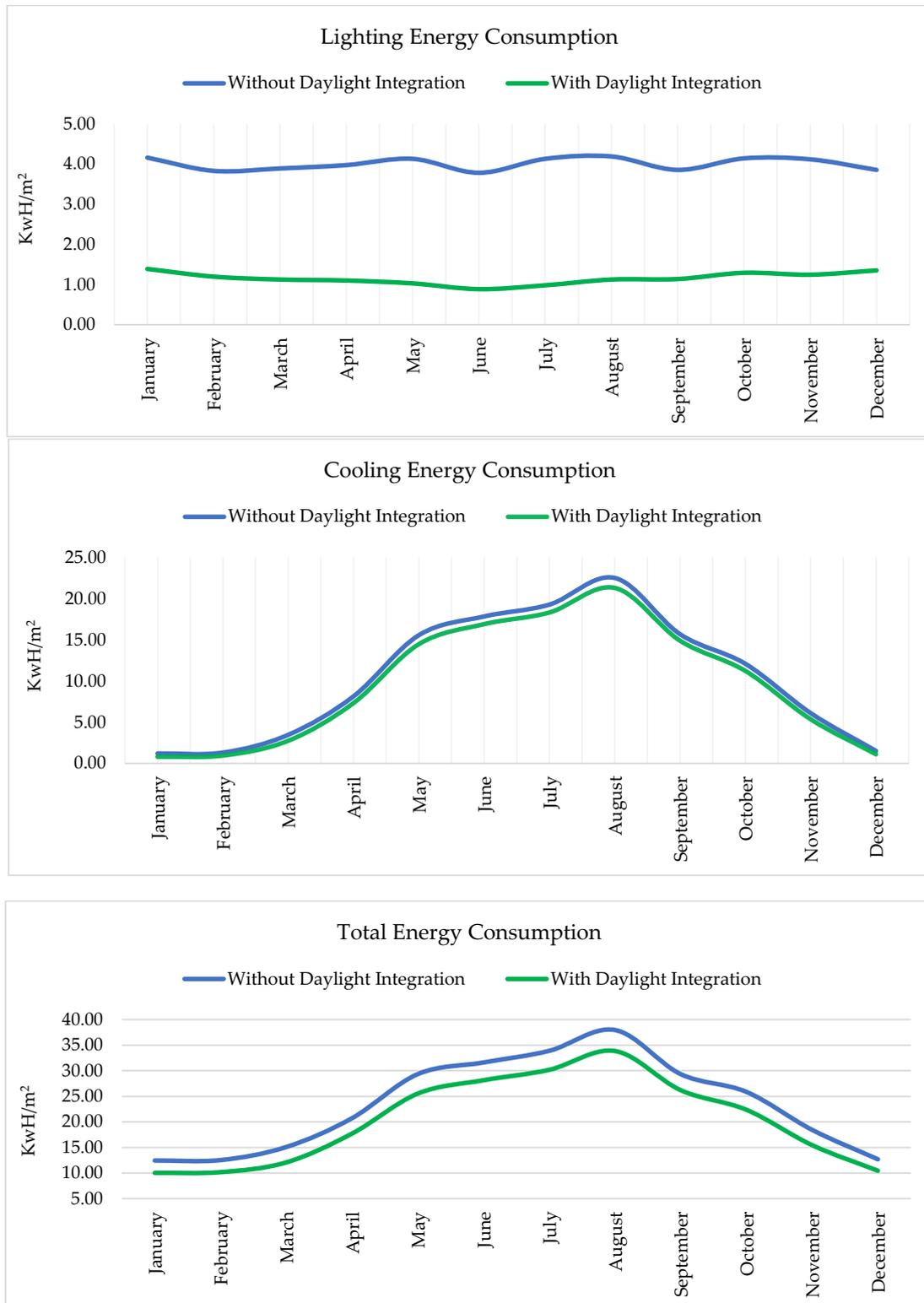
**Figure 4.** Total monthly electric energy consumption (lighting, cooling, and total) for modeled building with and without daylight integration.
