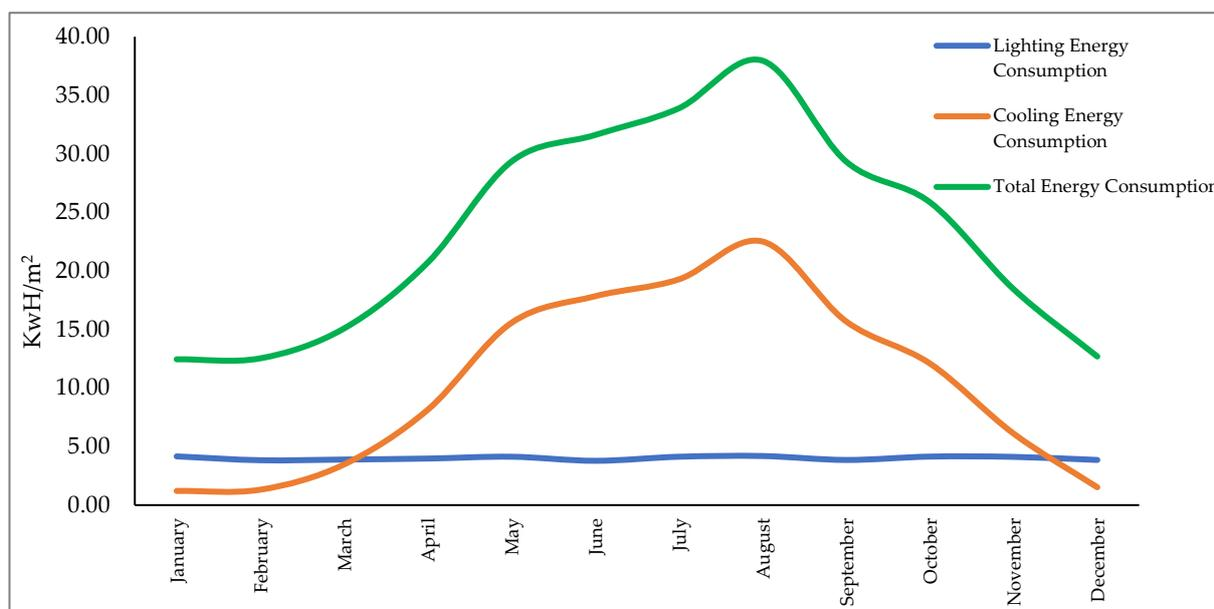
**Figure 2.** Electrical Energy Consumption for the modeled building over a period of one year.
