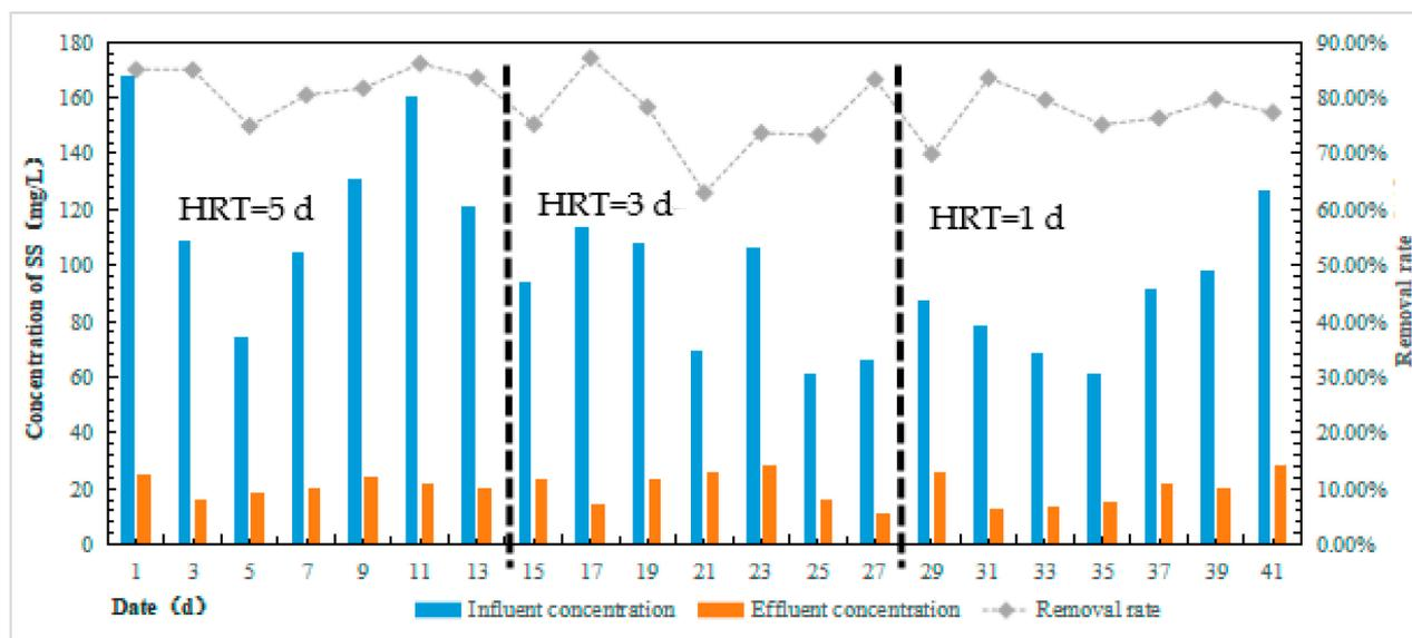
Figure 4. Effect of different HRT biofilms coupled with ABR septic tanks on SS removal.
