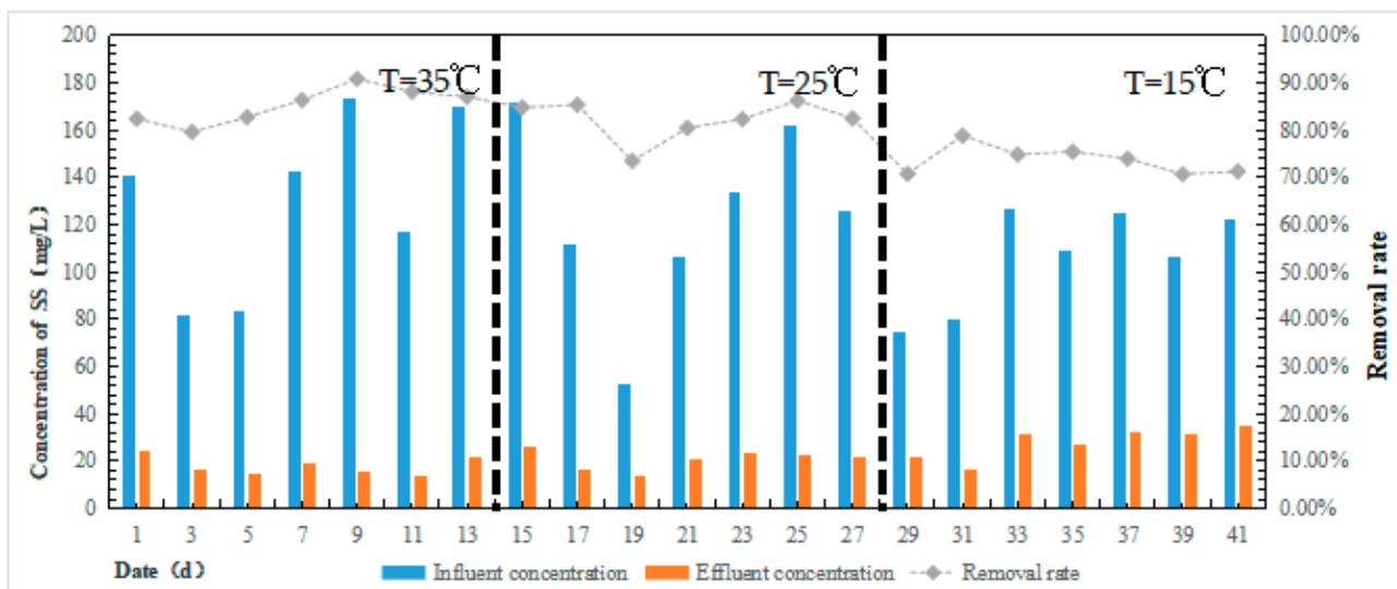
**Figure 8.** Effect of biofilm-coupled ABR septic tank on SS removal at different temperatures.
