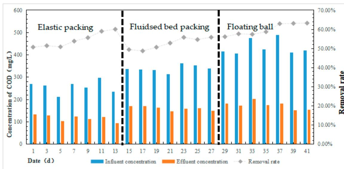
**Figure 11.** Effect of biofilm-coupled ABR septic tank on COD removal under different fillers.
