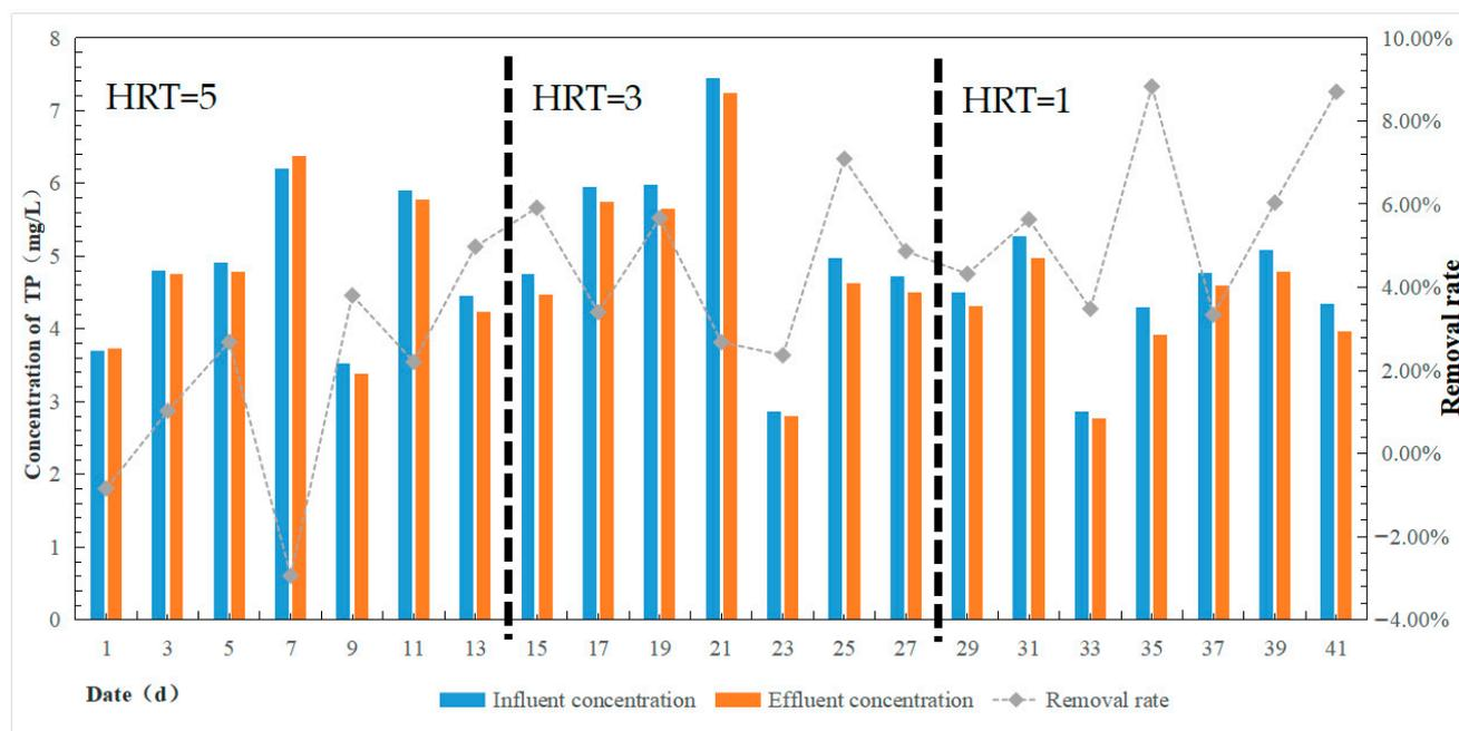
**Figure 6.** Effect of different HRT biofilms coupled with ABR septic tanks on TP removal.
