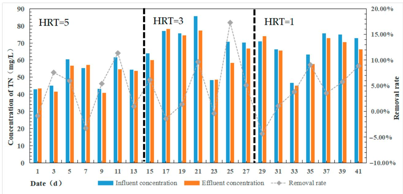
**Figure 5.** Effect of different HRT biofilms coupled with ABR septic tanks on TN removal.
