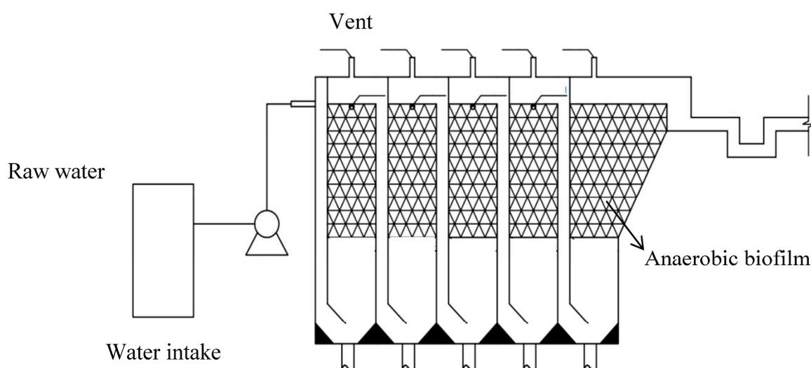
**Figure 1.** Diagram of the ABR setup.
