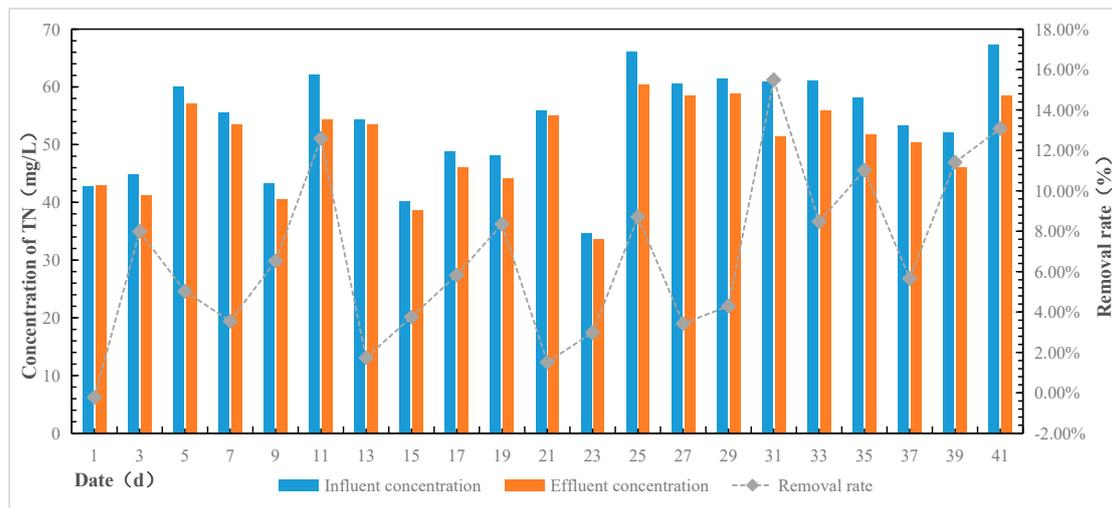
**Figure 13.** Effect of biofilm-coupled ABR septic tank on TN removal under different fillers.
