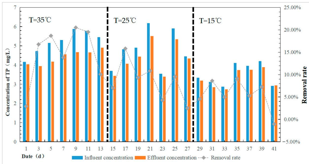
**Figure 10.** Effect of biofilm-coupled ABR septic tank on TP removal at different temperatures.
