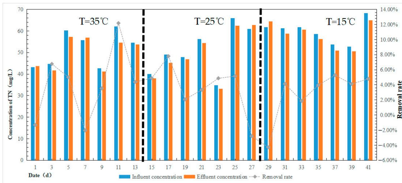
Figure 9. Effect of biofilm-coupled ABR septic tank on TN removal at different temperatures.
