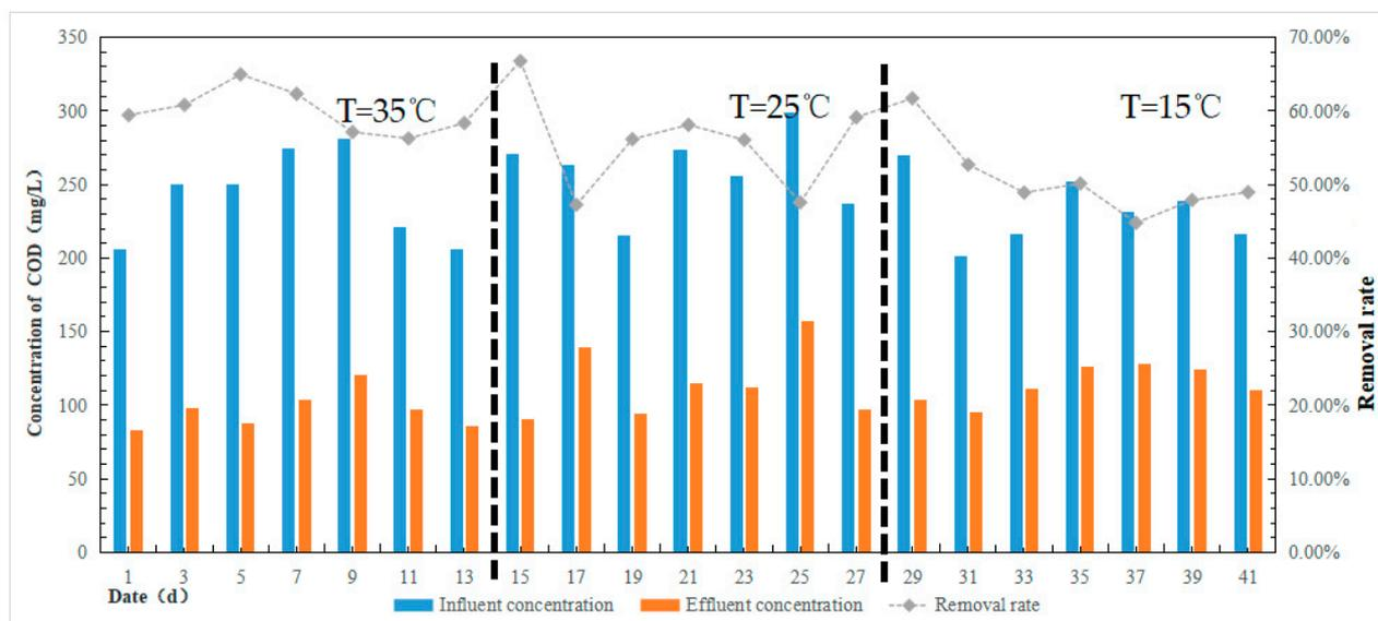
**Figure 7.** Effect of biofilm-coupled ABR septic tank on COD removal at different temperatures.
