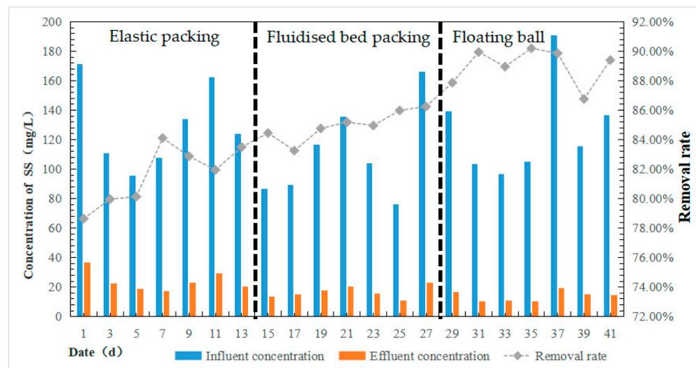
**Figure 12.** Effect of biofilm-coupled ABR septic tank on SS removal under different fillers.
