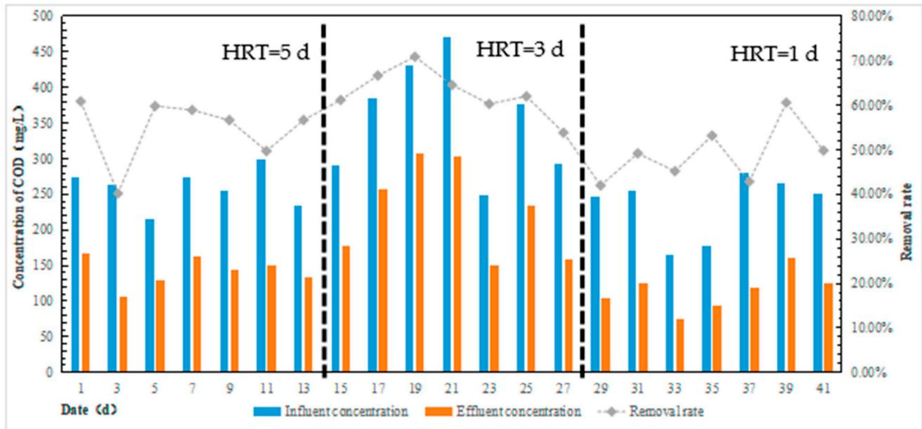
**Figure 3.** Effect of different HRT biofilms coupled with ABR septic tanks on COD removal.
