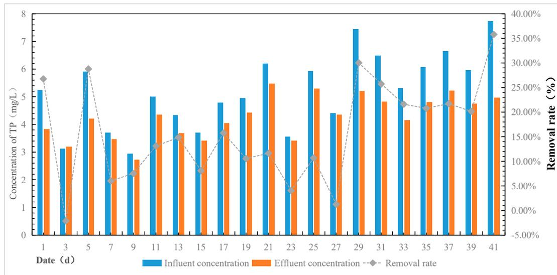
**Figure 14.** Effect of biofilm-coupled ABR septic tank on TP removal under different fillers.
