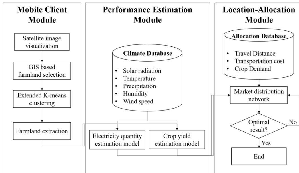
**Figure 2.** The structure of the decision support system for the APV system.
