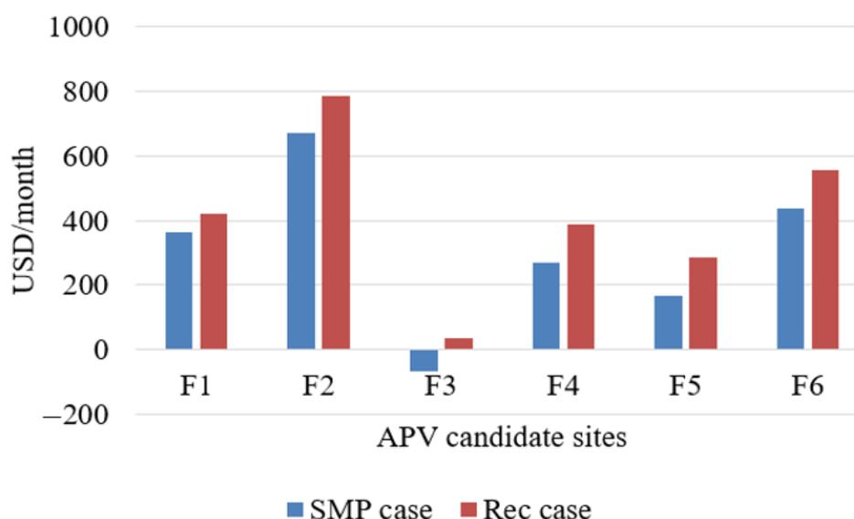
**Figure 9.** Total profits of bi-facial APV systems with a 25.6% shading ratio.
