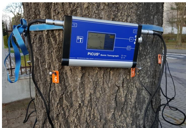
Figure 3. Acoustic tomograph CT scanner on a tree trunk (photo by M. Dudkiewicz).
